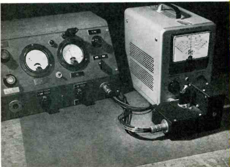
Fig. 10: Y_{12} (e) test set using the LC meter.
