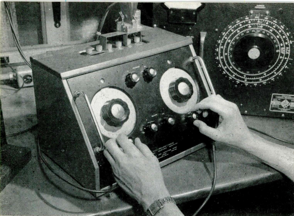
Fig. 1: Test set up: signal generator, Wayne-Kerr Bridge, receiver
