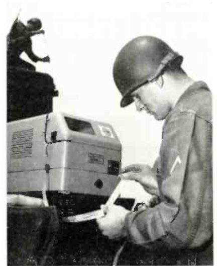
Signal Corps' new high speed teletypewriter stamps out messages at 750 words per minute.
