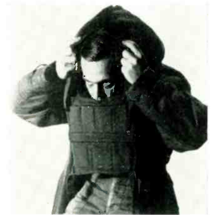
Battery vest is worn under a parka so that body heat will keep the chill out of the cells.
