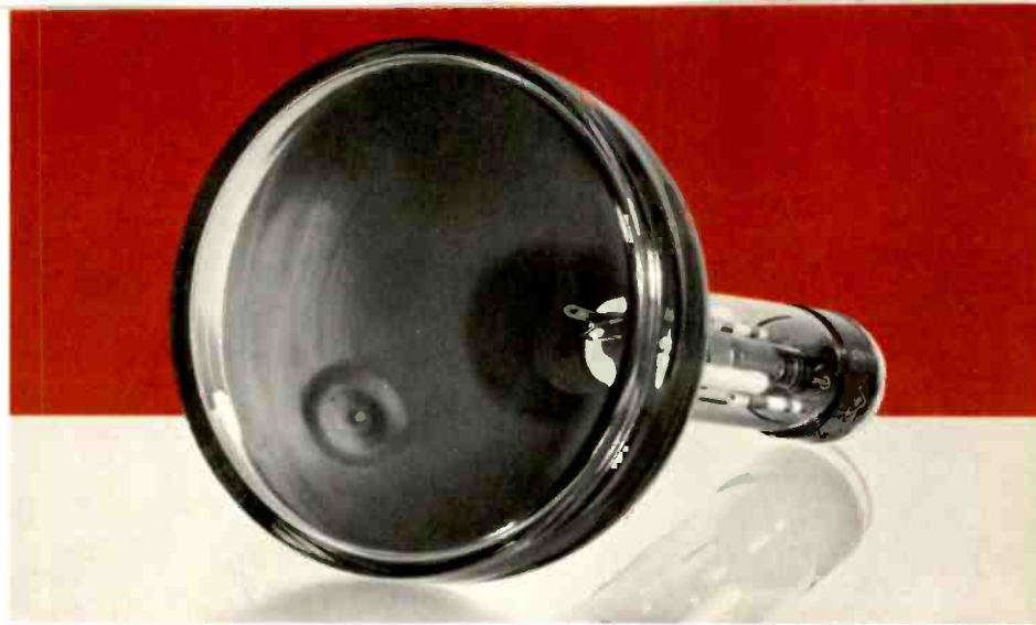
New five-inch experimental evaporated phosphor CRT
