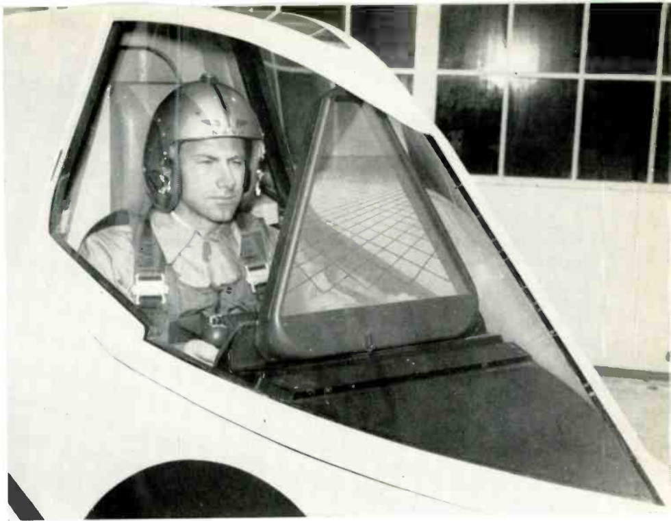
Mockup of cockpit shows thin, flat plate, transparent screen called contact analog.
