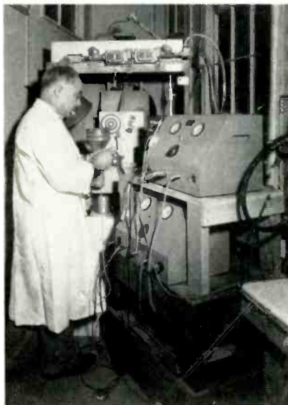
A gas-propelled abrasive removes the organic coating from this potentiometer winding.
