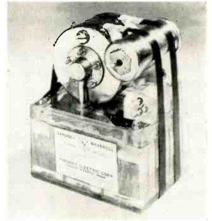
Fig. 3: A new automatic activation system lends itself to compact arrangements. Capable of being activated and operated in any position, it is used in ICBMs.
