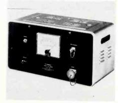
It has a meter and neon light for visual warning. Sensing unit can be either an alpha scintillation probe or a GM tube. The Victoreen Instrument Co., 5806 Hough Ave., Cleveland 3, O. Circle 235 on Inquiry Card, page 117
