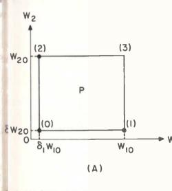
f. 4: (A) Space of operating points for a circuit with two aive elements—conditional stability; (B) and (C) contours guerated by the images of the vertices of P in the T-plane.
