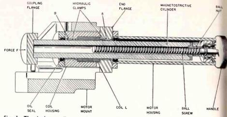
Fig. 1: The Inchworm linear actuator provides micro-inch dimensional control of delicate machine operations. One noteworthy application is in centerless grinders.
