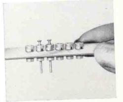
have a dc working voltage of 600 v. and are available 4.7  $\mu\mu f$  to 1000  $\mu\mu$ f. Operating temperature range is -55° C to +85° C. Cornell-Dubilier Electric Corp., S. Plainfield, N. J. Circle 203 on Inquiry Card, page 117
