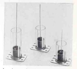
damping action in either direction. Two-way damping pots provide adjustable damping, equal in both directions. One-way damping models offer non-linear adjustable damping in the push or pull direction and fast reset. Weighing less than an ounce, they are available in various cylinder lengths and connecting rod spring gradients. Electric Regulator Corp., Pearl St., Norwalk, Conn.
