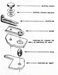
This positive, quick-action fastener was originally developed to hold airborne equipment with security – even under severe stress and shock of carrier-based aircraft operations – and yet permit equipment replacement in a matter of seconds.
