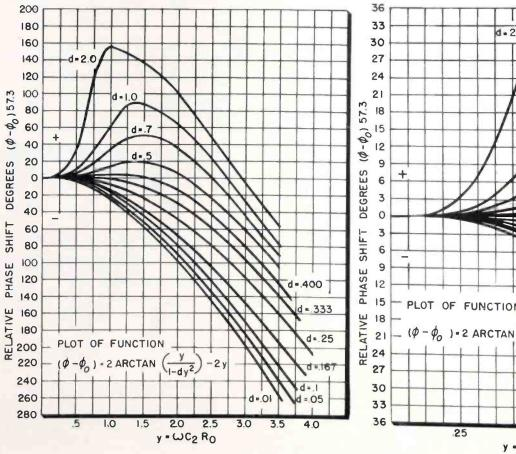
Fig. 1: Characteristics of all-pass lattices, function of "d" parameter.
