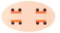
**D** Mica slots are designed with flat alignment surface and channel index to position grids with much greater precision. Closer element spacings are possible where extra Gm is required.
