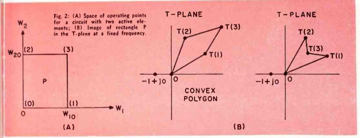
The functions  $F_1(p)$ ,  $F_2(p)$ , etc., are complex functas of frequency and are determined by the charsteristics of the active devices and the passive comfinents used in the interstage and feedback networks. The characteristic function is equal to the comminator of the gain function after it is normalled so that the constant term (independent of W) d unity.
