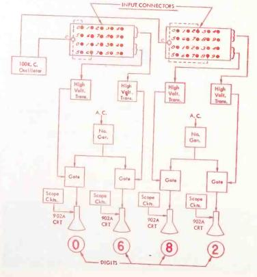
Fig. 2: Block Diagram, Hoffman digital readout Model DR-4C. used for each number in each digit to allow external control from pulse magnetic amplifier decade counters and other logical cir cuitry.
