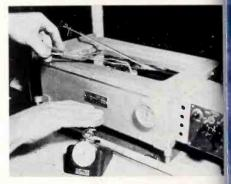
GE has developed a new copper clad glass expoxy laminate, Textolite 11558, reportedly capable of passing any dip solder specification in the industry. Here new laminate is tested in solder pot at 500° F.
