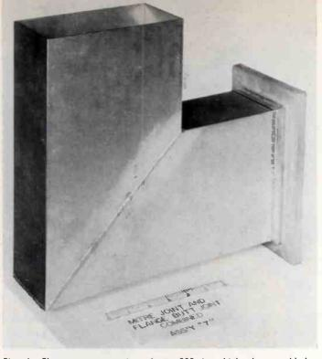
Fig. 4: Flange rear extension about .080 in. thick; butt welded.
