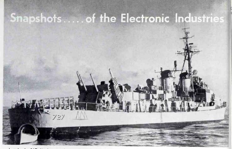
Launcher for RAT, Navy's new rocket-propelled, anti-submarine weapons system, is shown mounted on destroyer's aft 5-in. gun turret.
