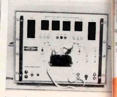
tween them, in a range from 1 ohm to 9.99 megohms. In addition to selecting either a 1%, 5%, 10%, or 20% nominal tolerance, it may be programmed to pass any value below or above a selected median resistance. The Robotester will perform a series of circuit checks automatically at 60 to 100 tests per minute. Punched tape provides a permanent test program. Lavoie Laboratories, Inc., Morganville, N. J.
