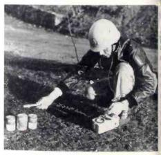
A N. Y. Civil Defense Warden checks food cans for radioactive contamination with new transistorized beta-gamma survey monitor manufactured by Universal Atomics Div. of Universal Transistor Products Corp.
