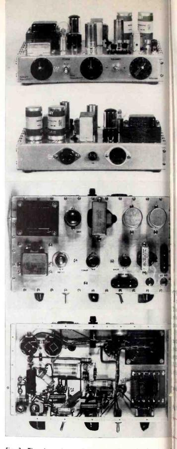
Fig. 3: The above photographs clearly indicate the location of components and controls of the prototype neon pulser. The author comments, "Major components in this pulser are substantially im-mortal, and should outlast the builder. The elecrolytic condensers, being rated at 450 volts, and used at less than 350 volts maximum have a life measured in years of use, and approximately two years idle."
