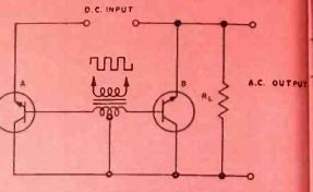
Fig. 3: Alloy junction transistors were most suitable for this switching circuit.
