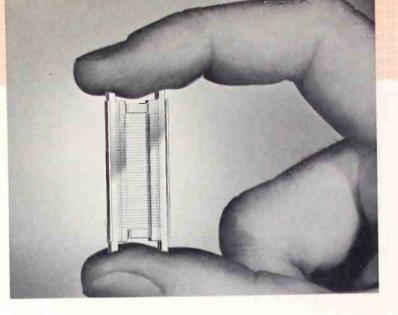
halves can be lined up. Perfect alignment means higher efficiency—greater flexibility in the selection of grid wire diameters for optimum performance.
