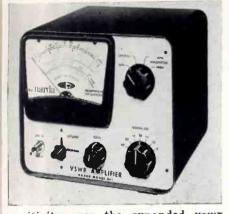
sensitivity over the expanded vswr scale and eliminates the need for switching attenuation range when going from normal to expanded scale. The noise level (less than .02  $\mu$ v. equivalent) and amplifier gain remain the same in the expanded position. Sensitivity is 0.1  $\mu$ v at 200 ohms, over the full scale. A protective circuit permits any switching operation or cable connection without danger to the bolometer. NARDA Microwave Corp., 160 Herricks Rd., Mineola, L. I., N. Y.
