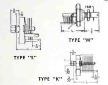
TYPE "S" CAPACITORS - The Type "S" Capacitor falls midway between the type "M" and "K" capacitors in physical size. Peak voltage rating 850 volts-plate spacing .013," other spacings available on special order. Square mounting studs tapped 4-40 on 17/32" centers.
