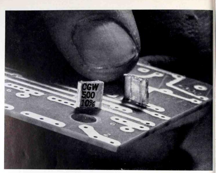
Truly sub-miniature, these capacitors were devised especially for printed circuits and automatic assembly. Since they retain all the properties of larger, pig-tail capacitors, they are well suited to general circuitry as well.
