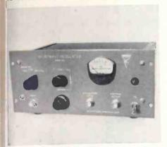
square wave modulated constant power source. The device itself operates at an audio frequency, hence, is completely independent of microwave power and frequency. By utilizing constant power, systems are more versatile and some measurements heretofore long and laborious, if not impossible, are done swiftly and with high accuracy. Brocker Labs., Dept. TT, P. O. Box 967, Sunnyvale, Calif. Circle 210 on Inquiry Card. page 117
