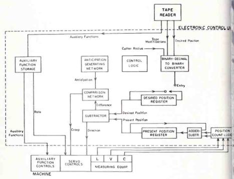
Fig. 11: Simplified block diagram shown here indicates the engineering philosophy underlyi the new tape-controlled machine shop used in production at Hughes Aircraft.
