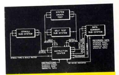
Fig. 2 (above) : Block diagram, automatic checkout equipment system.
