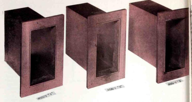
Fig. 1: These assemblies were torch brazed at the flange face.
