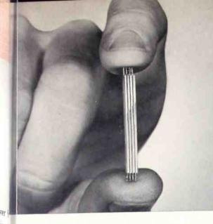
Many grids look like one! The inherent alignment capabilities of Sylvania's Framelok Grid are demonstrated by the ease with which the laterals of any number of separate grid
