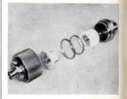
ing connector for 3 #8AWG wire, metal jacketed and mineral insulated cable. It is of special value where it may be necessary to frequently and quickly connect and disconnect large conductors. It has met environmental tests of 1.000° F., 100,000 ft. plus altitudes, 560 v. corona starting voltages and 960 v. flashover voltage. Concentric ring design eliminates alignment problems. AMP Inc., Harrisburg, Pa.
