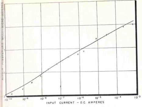
Fig. 8: The output vs the input characteristics of the logarithmic attenuator.
