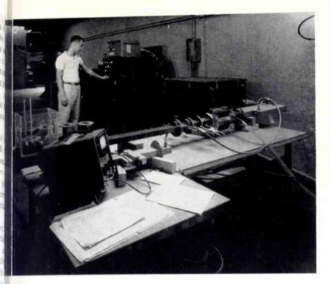
Fig. 1: With this test set-up, microwave ferrite isolators can be given realistic operating tests.
