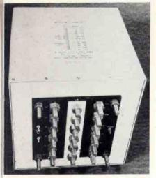
ninutes. Output voltages range from .2 to 230 v., and performance is naintained for any condition of loadng, from open circuit to 100 w. total f loads on all windings. Approxinately 500 separate conductors in eries and parallel combinations are ssembled in a Litzendraht type cable n order to achieve the proper degree f each winding among all the others. sborne Electronic Corp., 712 S. E. awthorne Blvd., Portland, Ore. Circle 242 on Inquiry Card, page 117
