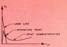
Fig. 2: Operating point must be in negative resistance region for oscillation.
