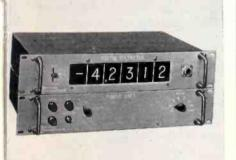
negohms on other scales. Automatic eatures include ranging, polarity and alibration. Stability is better than 1.01%. Electro Instruments, Inc., 3794 Rosecrans St., San Diego, Calif. Circle 243 on Inquiry Card, page 117
