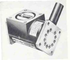
weighs 7 oz. and offers a frequency range of 9.2 to 9.4 KMC with isolation at 20 db min. and insertion loss of 0.5 db max. It incorporates a unique coaxial termination to permit both transmission and reception. Other features include: vswr of 1.25 max.; max. power absorbed in load is 12 w. and peak power at 10 kw. Kearfott Co., Western Div., 14844 Oxnard St., Van Nuys, Calif.
