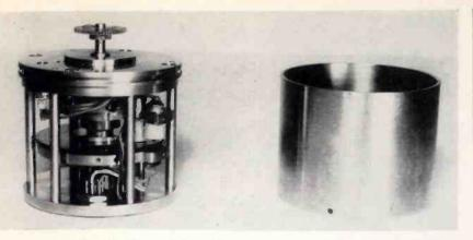
Fig. 1: The encoder with cover removed. It measures 3 inches in diameter by  $2\frac{1}{2}$  inches in length and weighs approximately one pound.
