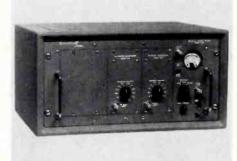
the new series features high sensitivity, reduced size and elimination of plug-ins. Model 7570 serves as a preamplifier of 1 mv. sensitivity in the 10KC to 10 MC range. Models 7571 and 7572 are heterodyne units with 10 to 110 MC and 110 to 220 MC ranges, respectively. Berkeley Div. Beckman Instruments, Inc., 220 Wright Ave., Richmond 3, Calif.
