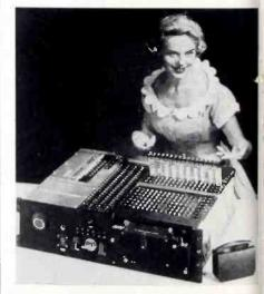
The "APAC" computer developed by Nortronics Div., Northrop Aircraft, is designed for airborne applications and features full transistorization. APAC (Airborne Parabolic Arc Computer) is packaged into 11/2 cu. ft., has magnetic memory drum.
