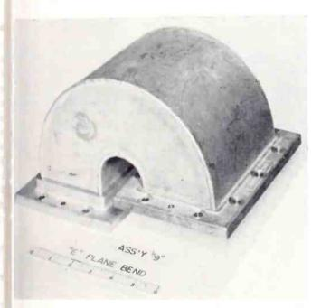
ig. 6: Slight gaps in waveguide wall at butt welds cause no trouble.
