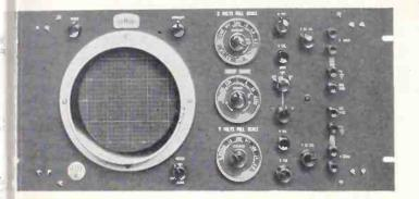
Identical in every electrical respect to its industry standard counterpart, the 401-R is physically rearranged for insertion into standard 19" relay racks. For quantitative and qualitative studies within the dc to 100 kc bandwidth, the 401-R offers important advantages in an easy-to-use configuration for panel operation. Some of these features... not available in other rack mountable units... are:
