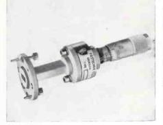
they are the most useful terminating impedances in waveguide measurements, apart from matched loads. The units consist of a section of waveguide in which a short-circuiting plunger can be moved by means of a micrometer drive. This is a non-contacting short of the two-section coaxial-filter type. Five types are available. Polytechnic Research & Development Co., Inc., 202 Tillary St., Brooklyn 1, N. Y.
