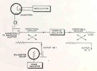
Fig. 3: Block diagram of test set for insertion loss and isolation measurements at rated power levels.
