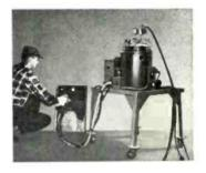
his heated pressure tank, with its heated hose and heated spray gun suc-
