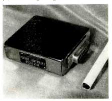
than 0.09 cu. ft. Power requirement per oscillator is 30 milliwatts and linearity is  $\pm 0.5\%$  of F.B.W. while drift is held to less than  $\pm 3\%$ . Dorsett Laboratories, Inc., Norman, Okla. Circle 202 on Inquiry Card. page 103
