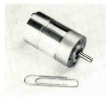
rated at 0.01 hp at 12,000 RPM, and Model 6A2 rated at 0.001 hp at 4,000 RPM. Model 6A2 is designed for continuous duty and requires a 0.22 amperes maximum current, while Model 6A5 is for intermittent service and requires 0.9 amperes maximum current. Western Gear Corp., P. O. Box 182, Lynwood, California.
