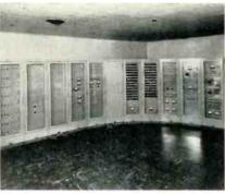
of Commutator, Analog to Digital Converter, Control and Timing Unit, Digital Tape Recorder and a unique built-in Test and Monitoring System. Beyond this point, the system may be expanded, using standard building block components, to fill virtually any data processing system requirement. Custom installations are available. Arnoux Corp., 11924 W. Washington Blvd., Los Angeles, Calif.
