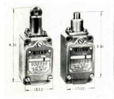
tact arrangements are double-throw 2-circuit, single - pole double-break. The electrical rating is: 10 a., 120, 240 or 480 volts ac; 0.8 a., 115 vdc. Micro Switch, Freeport, Ill.
