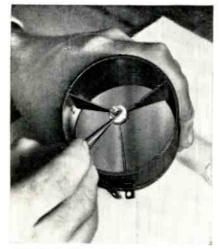
WEATHER EYES TO MEASURE CLOUD RADIATION. In the U.S. satellite, two "Weather Eyes" will peer from outer space at earth's cloud layer. Planned by the U.S. Army Signat Corps Engineering Laboratories and developed by the Perkin-Elmer Corp., Norwalk, Conn. to measure cloud radiation. these 4-ounce instruments are hardly larger than a pack of cigarettes. Each uses an f/0.7 mirror to pick up infrared cloud radiation and focus it on a tiny detector unit.
