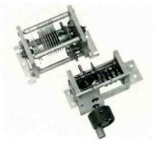
to within  $\pm 5$  parts in 10<sup>°</sup>. Features smooth operating precision bearings for maximum resetability accuracy; silver ground brushes provide secure grounding of rotor assembly;  $\frac{5}{16}$  in. dia. rotor shaft provides good stability and accuracy. The design and materials result in a temperature stable unit. National Company, Inc., Malden 48, Mass.
