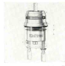
tube operation, is available. The RCA-7086 can also be used for gridcontrolled rectifier or inverter service. Capable of withstanding a maximum peak forward and inverse voltage of 650 v. at a maximum peak anode current of 400 ampere in intermittent service, or 160 ampere in continuous service. Radio Corporation of America, Harrison, N. J.
