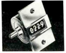
counters are available in a range of 3-6 figures. The driveshaft is 1/8 in. diameter and can project from the left or the right hand end of the case. When additional actuation is necessary as count is registered, the driveshaft can project from both ends of the case. Revolutions may be counted at a maximum of 1000 per minute. Technicraft, 6221 Ridge Ave., Phila-
