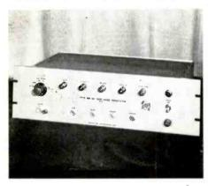
The markers and sine wave are derived from a 1 MC crystal-controlled oscillator. Dimensions are: 5<sup>1</sup>/<sub>4</sub> high, 19 wide, 9<sup>1</sup>/<sub>4</sub> in. rack depth, 11 in. overall depth. Available with a temperature-stabilized crystal oven installed. Tektronix, Inc., P. O. Box 831, Portland 7, Oregon.
