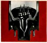
1. "Old" Hand-Tip-Cross section of earlier style base showing seal obtained employing previously used hand tipping
