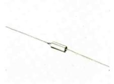
rosion. Capacitors have good stable capacity and dissipation factor over the range from  $-80^{\circ}$  to  $+85^{\circ}$ C. Shelf life is indefinite. They have axial lead construction, with hermetic glass-to-metal end seals. Leads are approximately 142 in. long-of .020 in. wire, nickel-tinned. Available in standard EIA capacities. P. R. Mallory & Co., Inc., Indianapolis, Ind.
