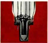
3. "New" Automatic Tip-Cross section of rigid pin base used on 110° nicture tubes
