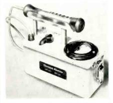
a transistorized radiological survey meter, a transistorized dosimeter charger, and three safety dosimeters. The all-transistorized survey meter, Model UAC 700, is a rugged, lightweight unit that operates from standard flashlight cells for more than 250 hours of continuous use. It meets military specifications. Universal Transistor Products Corp., 143 E. 49th St., New York 17, N. Y.
