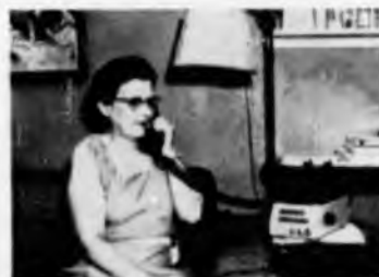
Phone service for isolated rural areas becomes practical with this new push-button dialing radiotelephone developed by Motorola. System uses automatic exchanges.
