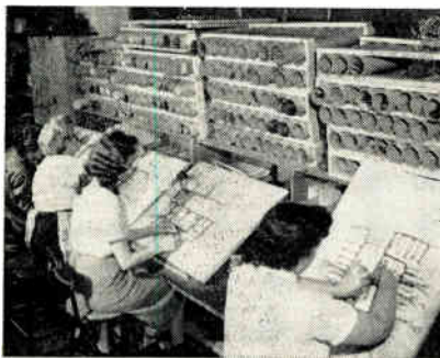
Wiring of intricate harnesses is one of the sub-assembly production techniques employed at Telectro Industries Corp., L.I.C., N. Y. Harness shown is for tape transport.
