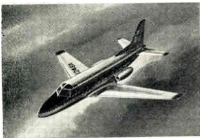
The "Sabre Liner," a 500 mph utility craft, will be built by North American Aviation for the military. Power will be supplied by two GE J-85 turbo jets, on aft fuselage
