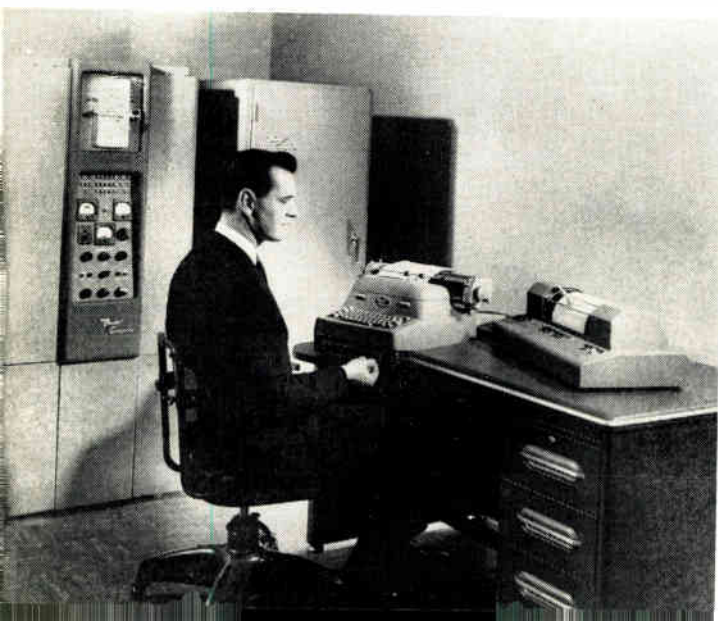
Fig. 1 (left): From left to right—Bendix G-15 computer, digital differential analyzer, input output typewriter, X-Y plotter.
