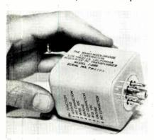
in epoxy resin and sealed. Operates over ambient temperature range of -55 to 71°C. Unaffected by extremes of shock and vibration. Package operates on 24 to 32 vdc. input and delivers 900 vdc. at 30 ma within 3%. Output ripple is regulated within 3 v. peak to peak. The entire unit is integrated in a 2 x 234 in. package. The Ramo-Wooldridge Corp., P. O. Box 8405, Denver 10, Colo.
