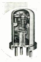
Polarized operating characteristic of this magnetic d-c Relay makes it ideal for use as a null detector in ordinary bridge circuits. It can operate directly from a thermocouple or photocell. Both coils brought out to separate pins in base make it easy to calibrate and overhaul and versatile to apply. Hundreds of thousands of these relays are now in use in airborne control equipment.
