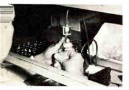
Visual inspection—visual inspection criteria as outlined in MIL-E-1C is applied to Guided Missile Tube production. This highly stringent and definitive spec helps to insure optimum reliability.
