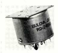
warm-up requirement. The 10 and 15 crystal oven will stabilize within  $\pm 2^{\circ}$ C over an ambient of  $-55^{\circ}$ C to below reference temp. Available in units housing a 1, 2, 10 and 15 crystals. Operating voltage for the 10 and 15 crystal units is 6-115 v. ac or dc. The one unit oven is available from 6-24 v. ac or dc. Bulova Watch Co., Electronic Div., Woodside 77, N. Y.
