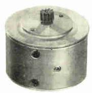
115V. 400 CY. 10 WATTS SPEED: 12000 RPM (N.L.) TORQUE: 0.5 in. oz. (stall) SIZE: 1.6" DIA. 1.0" L.
