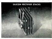
These units consist of hermetically scaled junction diodes mounted on copper cooling fins, stacked to include the interconnections required for specific circuits. Junction ratings: 1.25 amps. DC output; 70 to 350 AC input volts rms. Request Bulletin SR-137A.
