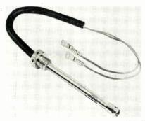
cision tolerances are 0.05%, 0.1%, 0.25%, 0.5%, 1% and 3%. Resistor is wire wound. The resistor element is surrounded by a resilient material and inserted into the protective brass tubing. Shock absorbing material completely protects the element. Applicable types conform to MIL SPEC MIL-R-26-C. Maximum operating temperature is 275°C. Dale Products, Inc., Columbus, Neb.
