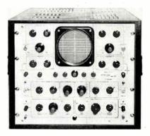
10 kv acceleration potential and transistorized multi-vibrator. Time base is separate or common as selected. Triggering is either internal or external. Electronic Tube Corp., 1200 E. Mermaid Lane, Phila. 18, Pa.
