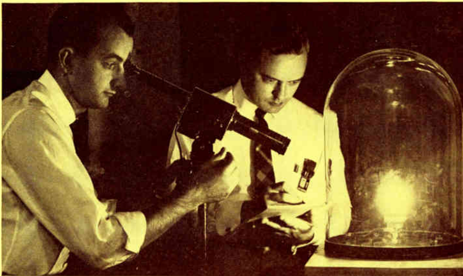
Checking a GL-6942 for operating temperature (optimum relationship between cathode emission and cathode life). Increasing power is fed into tube filament until cathode glow matches color of the element in the optical pyrometer, calibrated for 1950K—the optimum figure. Thoriated tungsten for the cathode permits high-output service with long tube life. See further GL-6942 story on next page, describing tube and its applications.
