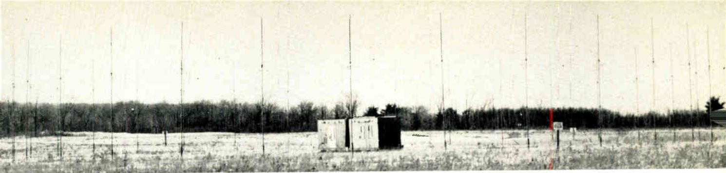
Fig. 1: Doppler-type direction-finder, AN/TRD-8, uses 31 antennas in circular array. Shelter in middle houses equipment.
