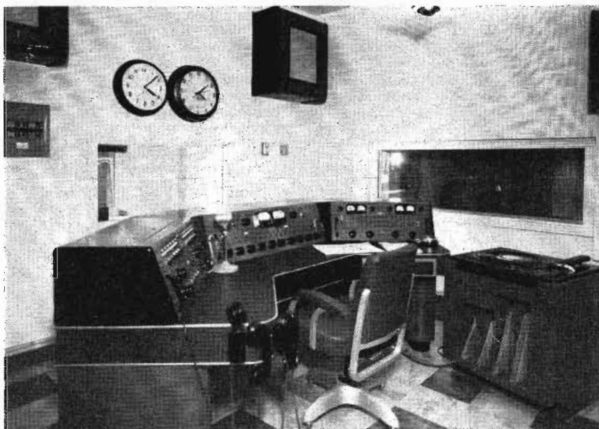
Three Collins consoles handle all the speech equipment switching and preset selecting of studios. Left to right: telephone, line, master control and preset switching consoles
