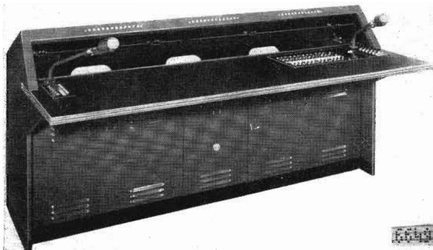
Fig. 7: (Below) Program director's console contains program monitors and mounts relay switching panel for studio control system
