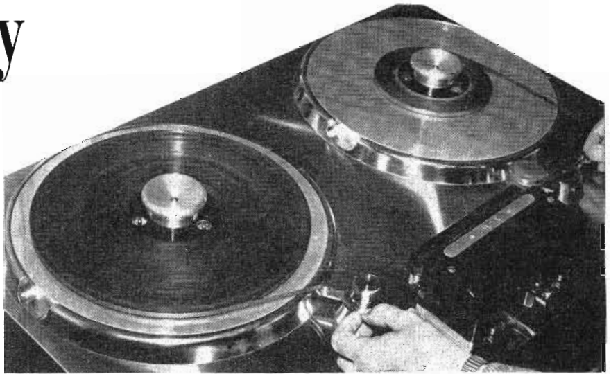
Professional tape recorder (Ampex), using low coercive force tape, operates at 30 in/sec
