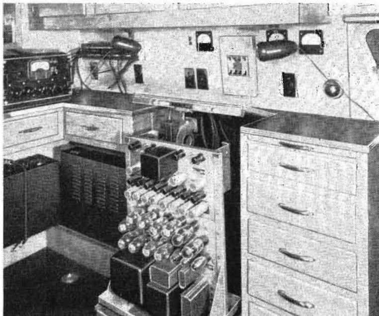
(Left) Camera chain storage unit cabinets are made of solid oak, fully lined with foam rubber for shock protection. Distribution amplifier can be seen at right in lower corner. (Right) Close-up view of the video distribution amplifier, uncovered and pulled forward for inspection
