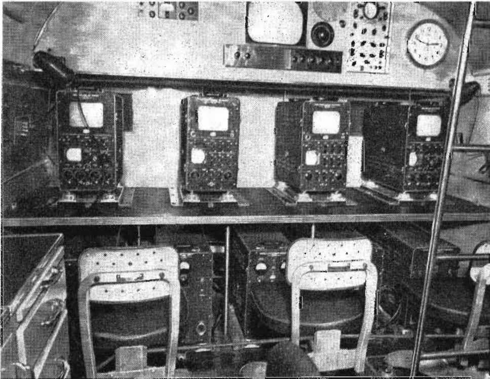
Photo showing equipment arrangement at camera control and video switching positions Author checking power supply unit which slides out on a track for easy accessibility
