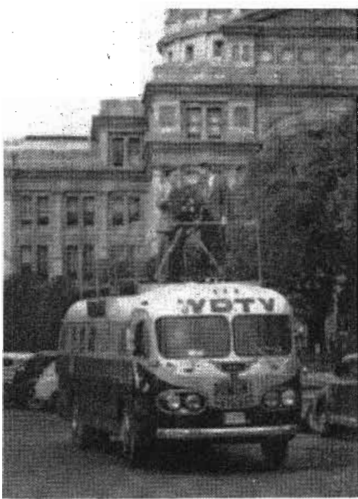
Pickup being handled with truck in motion using self contained gas-engine generator. State capitol at Austin, Texas in background
