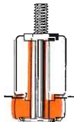
Silicone gaskets and porcelain stand-offs used with capacitors rated 2500-v to 5000-v d-c.
