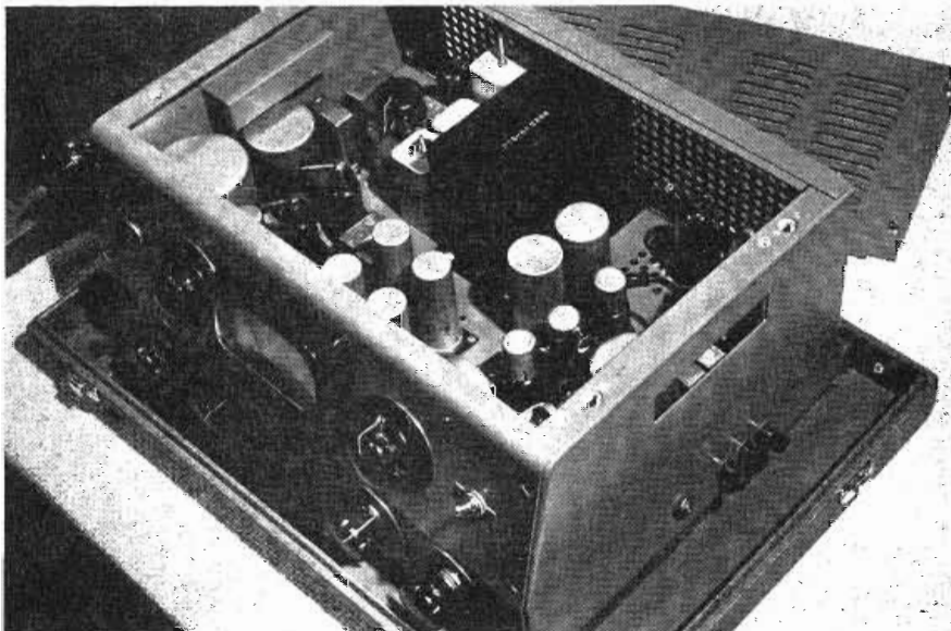
Fig. 5: Internal constructional layout of recording amplifier console and its controls
