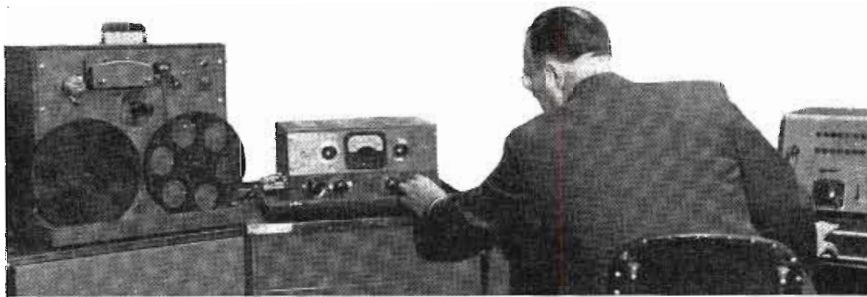
Fig. 1: Overall arrangement shows how recorder can be placed in control room in such a manner as to permit airing or recording of program material on tape by the operator
