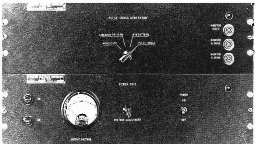
Fig. 10: Photograph showing the front panel and controls of the pulse cross generator
