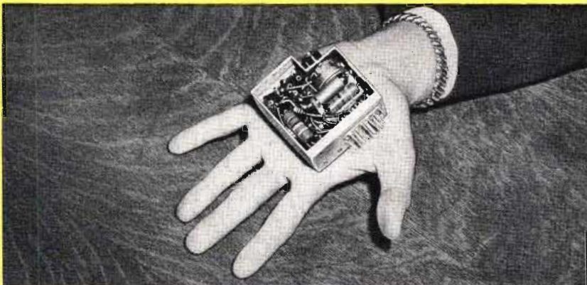
The trend towards subminiaturized construction is being applied to many types of present-day equipment by Philco research and development engineers. This model of a plug-in unit provides a sweep generator circuit that is readily replaceable.
