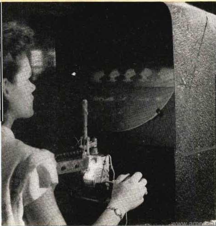
Production type comparator test equipment checks RF turret tuner switch contacts before mounting sub-assembly on receiver chassis
