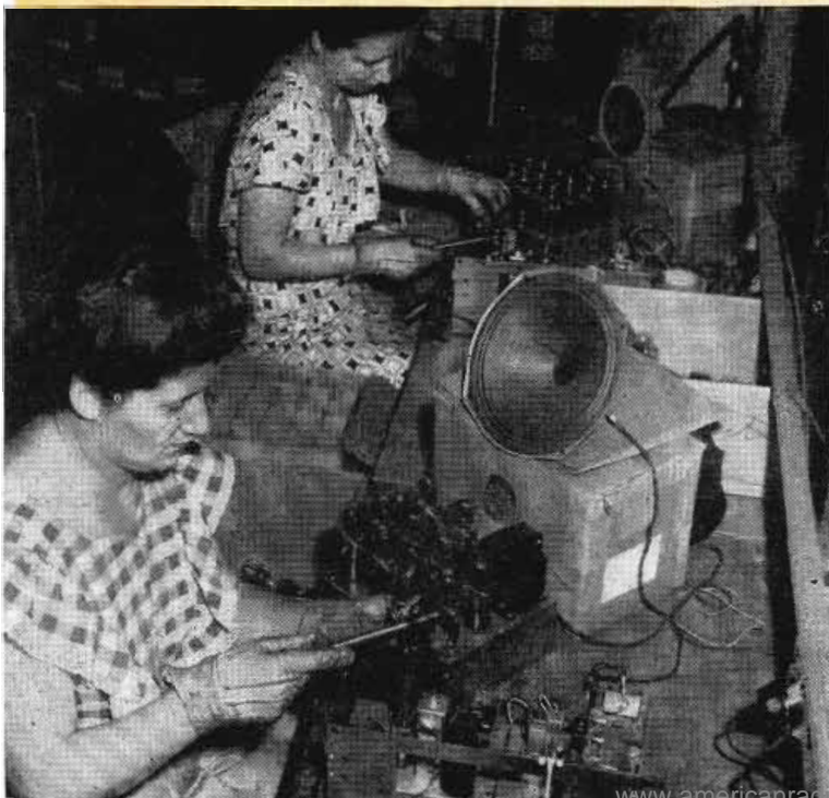
New tubes undergo an actual operation test in radio receiver chassis before they are released as production components
