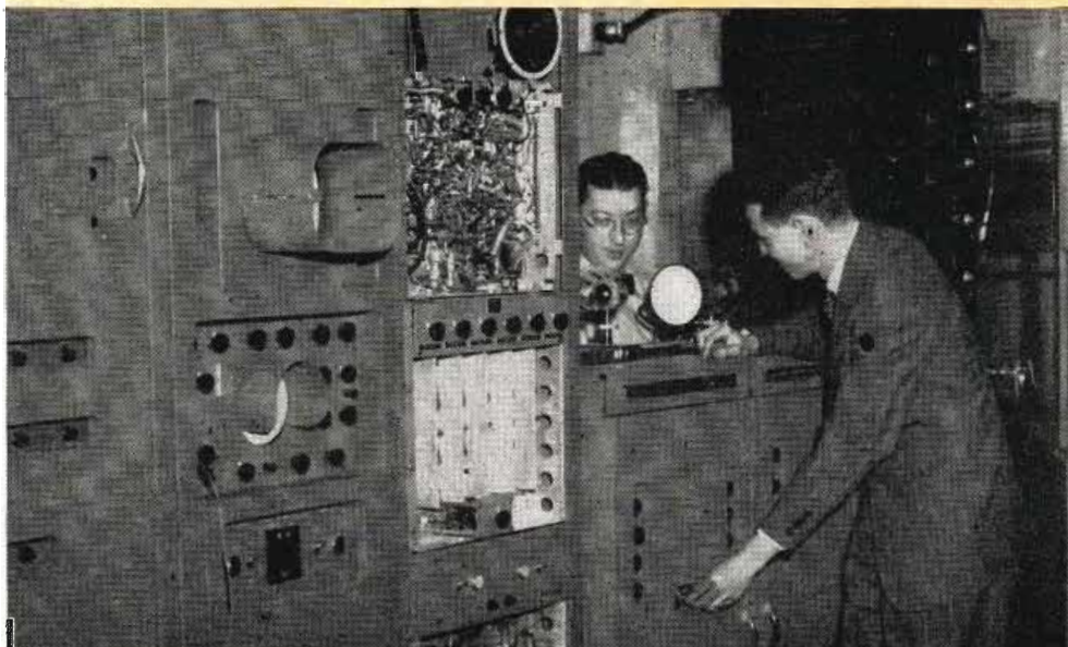
This flying-spot scanner, used to provide TV pictures of varying contrast range, is typical of aids to video development designed by the test-equipment section of the Research Division
