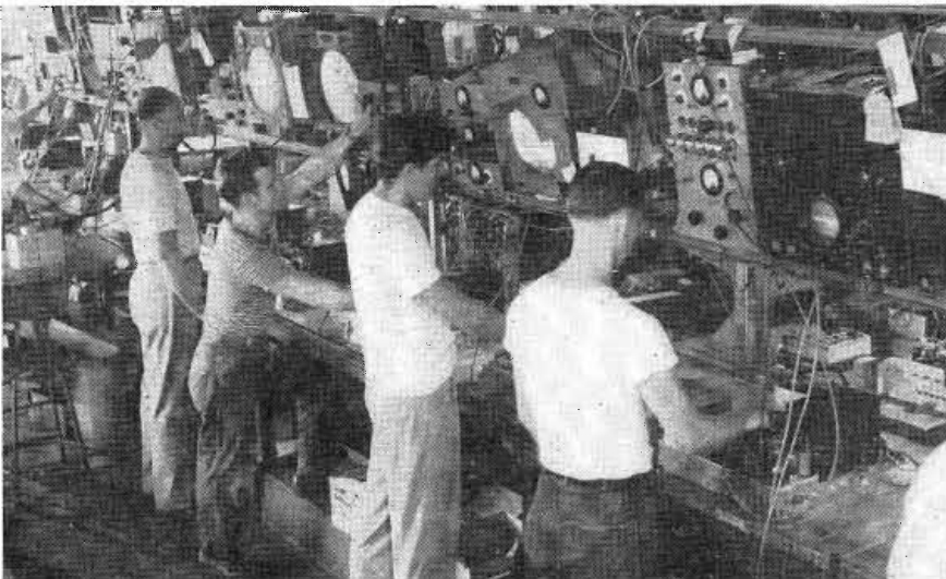
Test equipment mounted at eye level above chassis conveyor facilitates set alignment. Celluloid masks on oscilloscope screens show desired curve shapes
