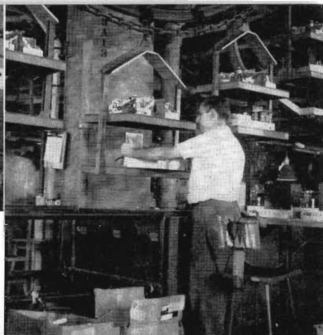
After alignment, chassis are loaded on a monorail conveyor that transports them to second floor for cabinet mounting
