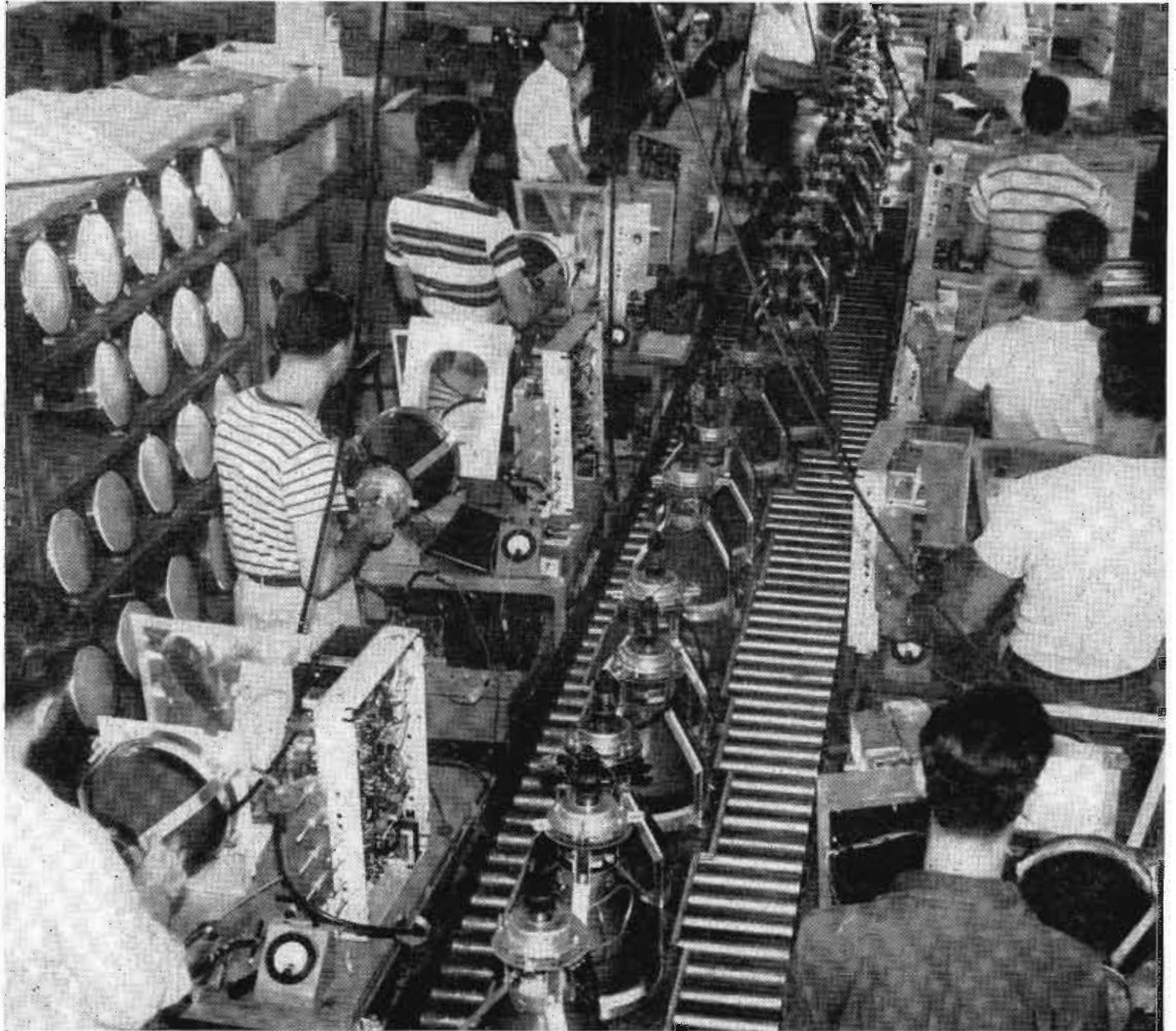
Cathode ray tubes, ready for mounting in new television receiver cabinets, being tested enroute to the main production lines.
