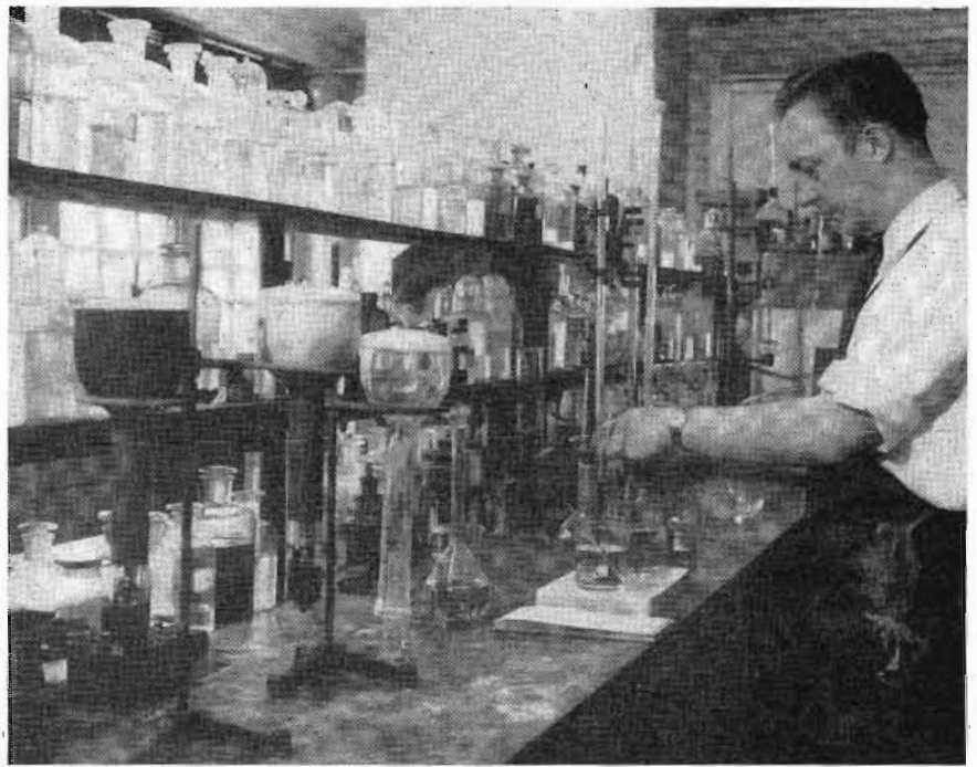
Chemist preparing a new phosphor solution for coating viewing screen of an experimental cathode ray tube. 4-in. projection tubes at left are in various stages of development
