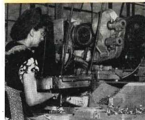
TV components that are sub-assemblies are constructed on auxiliary production lines. Riveting tube sockets and terminal strips onto the main chassis is primary operation
