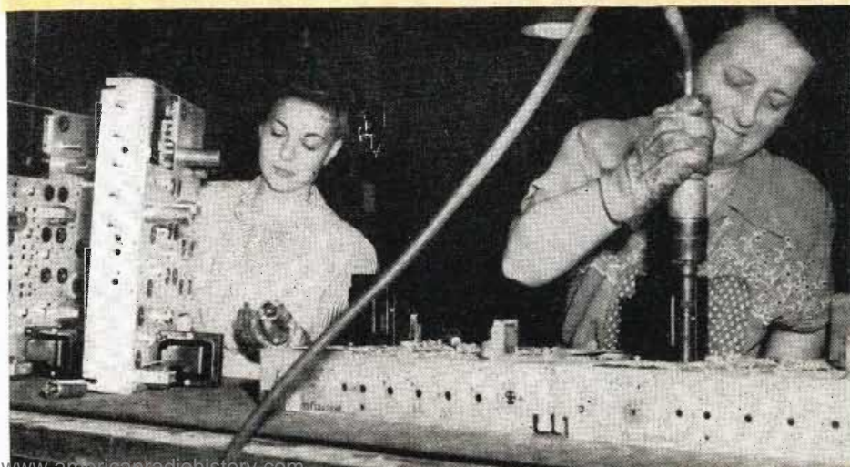
Larger components, such as chokes, power transformers and electrolytics, are then mounted. Small resistors and coupling capacitors are added during the various wiring operations.
