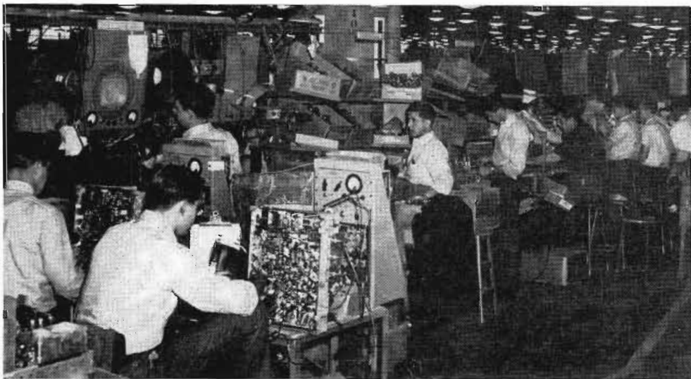
Trouble shooting area located near preliminary "hot" or signal test point. Chassis with any faulty circuit constants are intercepted before proceeding for final test operations
