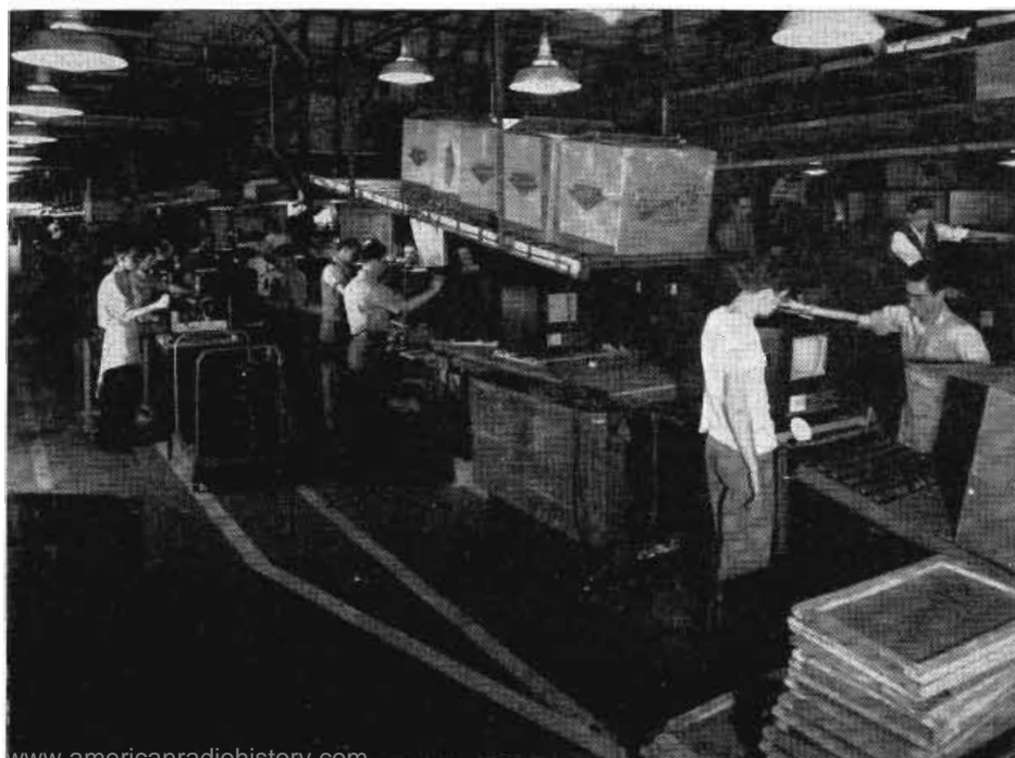
Shipping cartons traveling on an overhead conveyor, meet the finished instruments at the end of the production line. With sealing of the carton, set is ready for shipment
