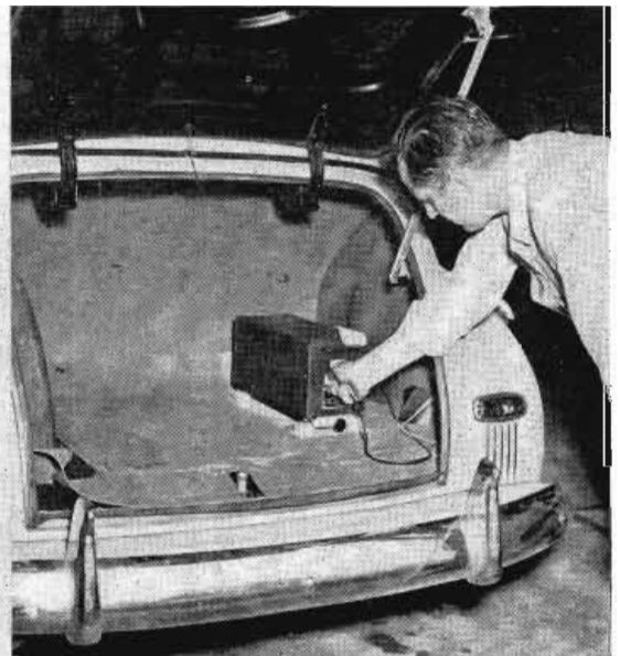
Transmitter-receiver installation in rear. A thin co-ax cable leads roof-top antenna
