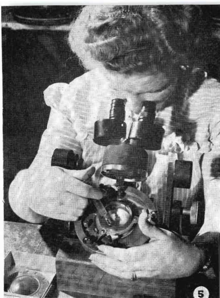
Fig. 5: Voice coil of Western Electric's 713 receiver, a component of the 757A loudspeaker, is attached to diaphragm at Burlington plant. As in winding of voice coil for the 756A, assembly is aided by use of high power microscope
