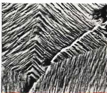
▲An example of Electron Microscope's magnification 46,500X of chrome iron by replica and shadowing. Used by courtesy of Dr. Wyckoff and Dr. Williams.
