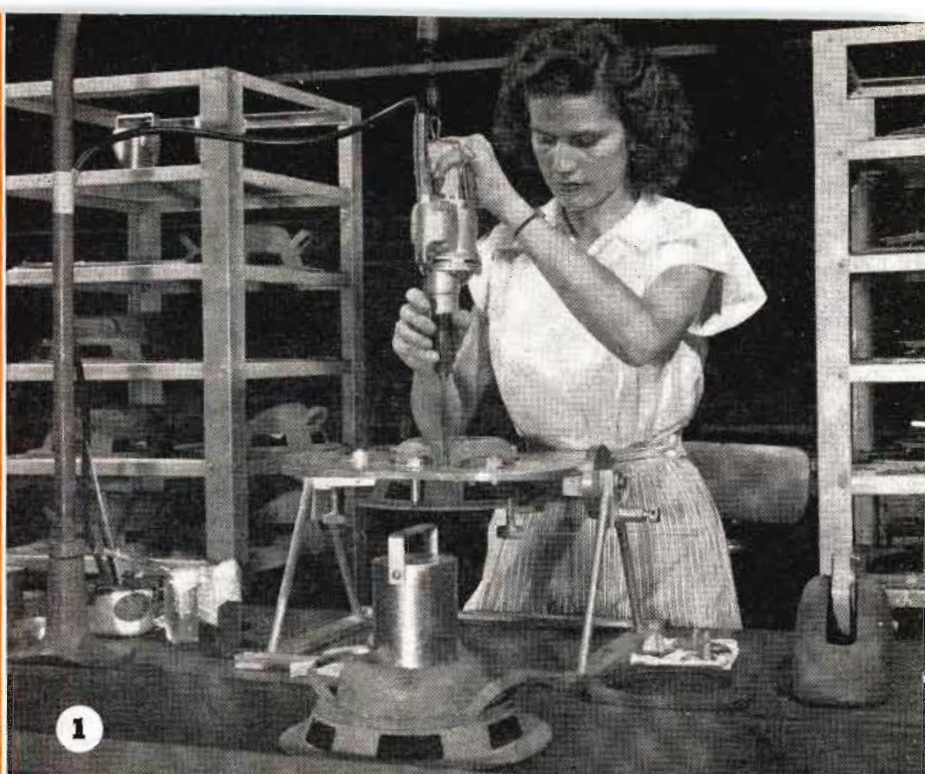
Fig. 1: Frame of Western Electric 756A loudspeaker is mounted in assembly jig at the company's Burlington, North Carolina, plant. Power tool is suspended by a spring mounting over the work area, expediting and facilitating the operation
