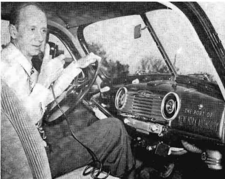
VHF equipment in this Port of New York Authority car assigned to Idlewild operates on 121.9 mc. Control unit with microphone is mounted under dashboard
