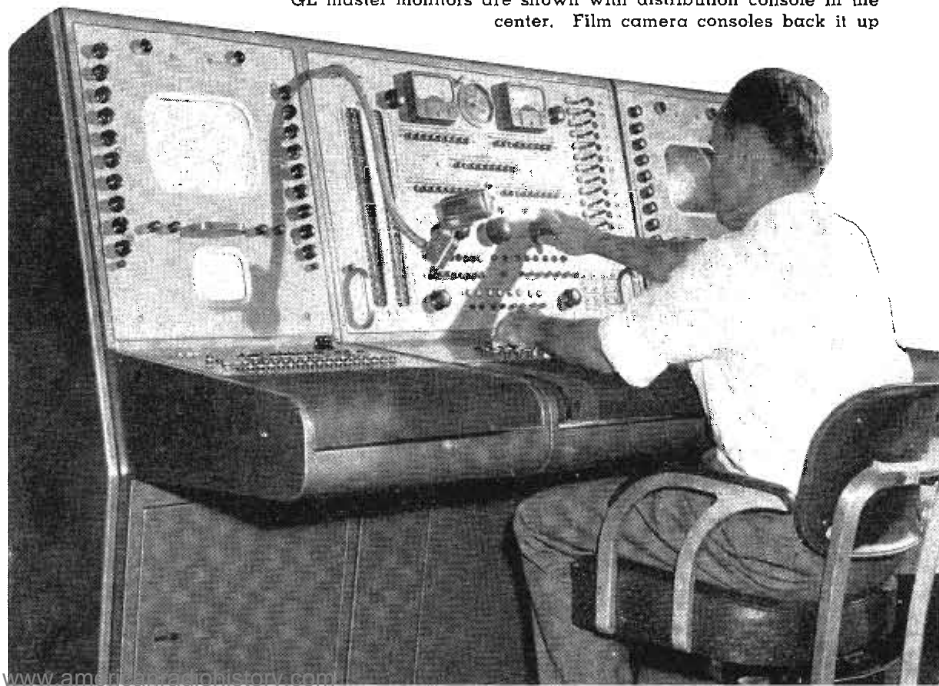
GE master monitors are shown with distribution console in the center. Film camera consoles back it up
