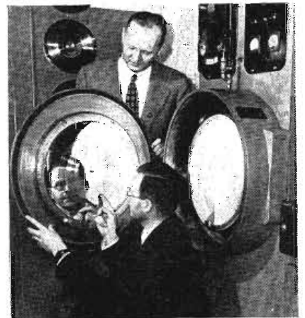
Dr. Peter Goldmark, CBS Director of Engineering (kneeling) and William Bachman, Director of Research for Columbia Records, examine chamber for gold coating master record
