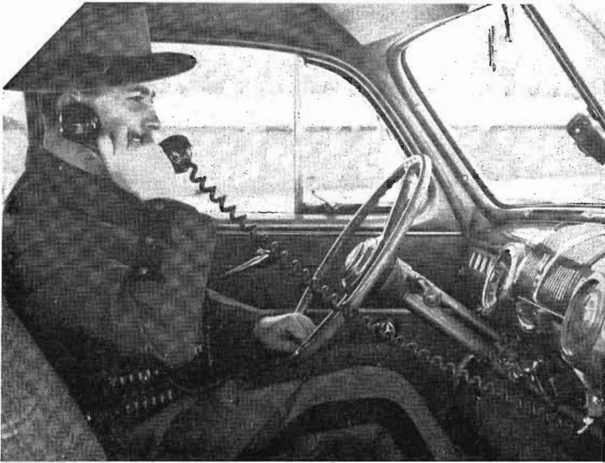
Above: Showing state trooper transmitting from patrol car with 2-way mobile installation
