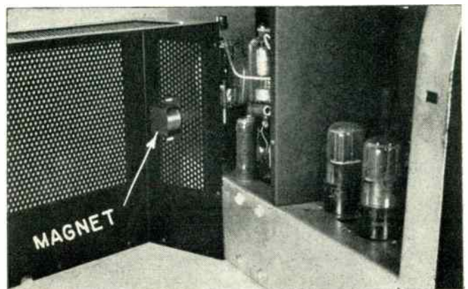
Fig. 4: View of horizontal deflection amplifier and fly-back supply of receiver showing magnet for oscillation suppression bolted to cover which, when in position brings magnet against horizontal amplifier tube
