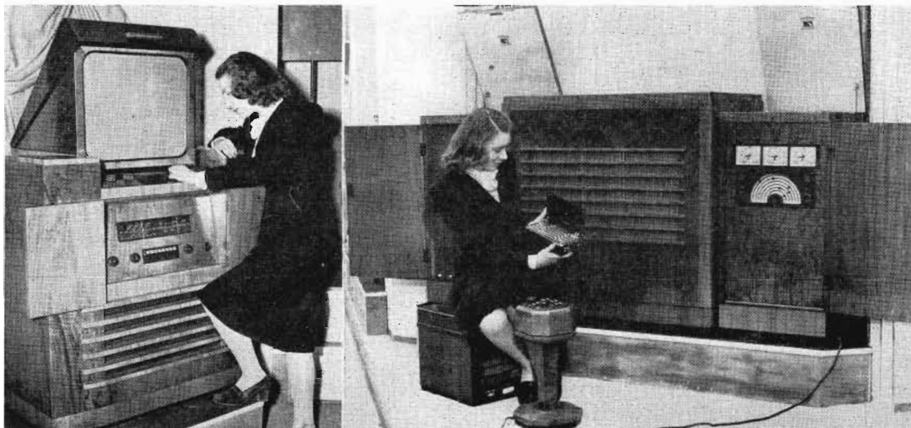
At left is shown one British version of a large-screen (16x20 in.) home projection television set which also incorporates an all-band AM receiver. Model at the right is a 43-tube remote-controlled console containing an all-band receiver as well as an automatic phonograph. Set will automatically switch itself on to any of three preselected programs at predetermined times. Girl is holding a personal portable which uses all miniature tubes
