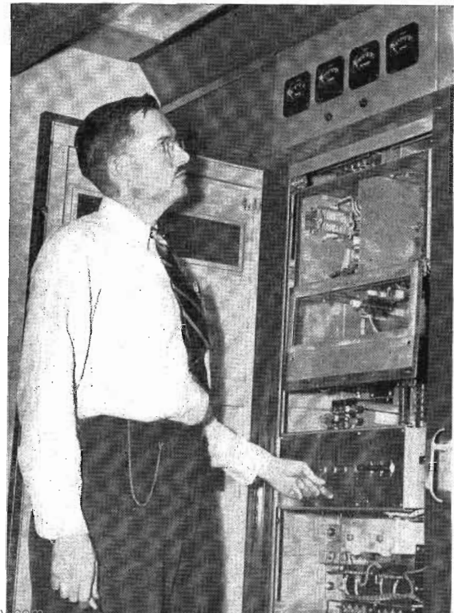
WRC-FM, opened simultaneously, has an RCA type BTF-3B transmitter, uses the same antenna tower, power of 15 kw
