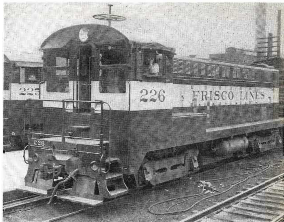
Bendix VHF train radio in use on the Frisco lines at Springfield, Mo. "Wagon wheel" antenna appears over engine cab
