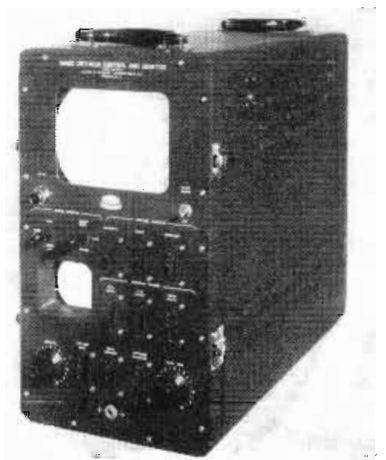
Fig. 8—Camera control and monitor unit
