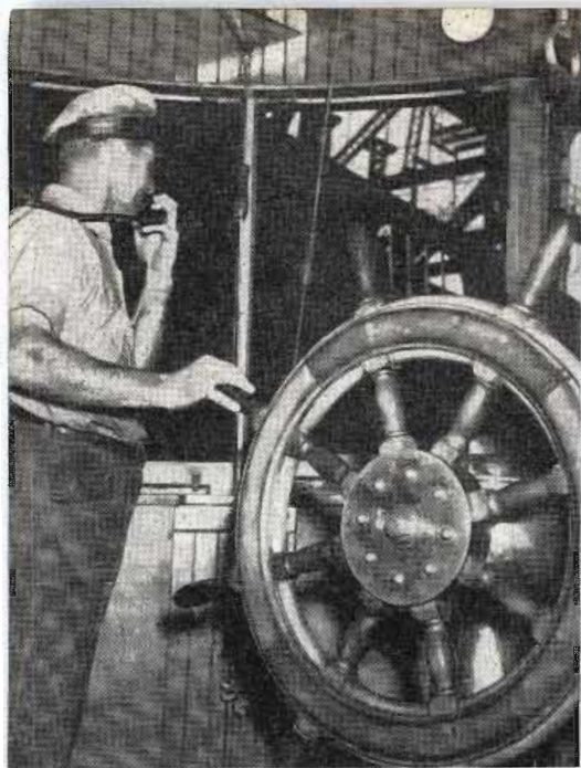
Bendix VHF space radio communications on C&O tug at Newport News with mate talking to boatmaster at off-shore end of pier
