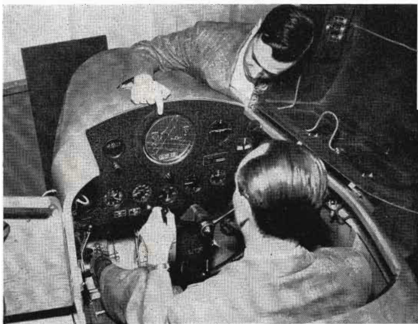
Typical installation of an RCA Teleran receiver in the cockpit of a flight simulator. Equipment gives the pilot all needed route, traffic and weather information on a single image screen on instrument panel
