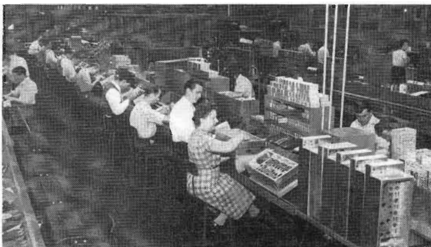
Assembly line in the Bendix Towson plant, showing production of VHF railroad equipment from "raw" chassis to finished product
