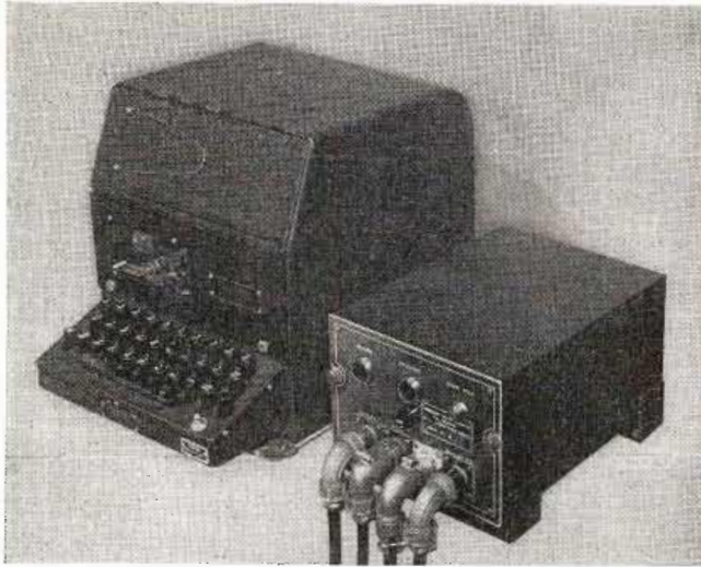
New teletypewriter with associated converter-control unit Interior view of converter-control used with radio circuits
