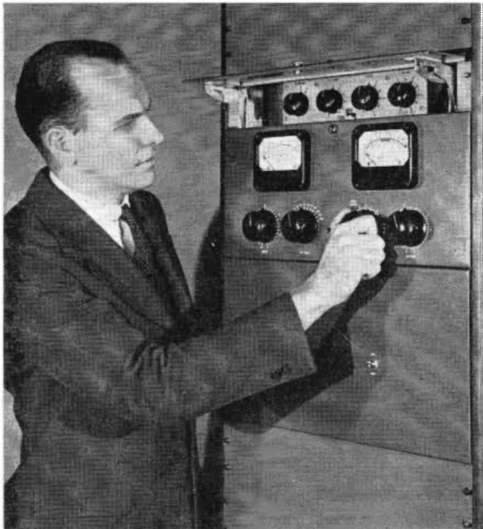
• View of front panel of the gain - adjusting amplifier in its standard cabinet with the author at the controls •
