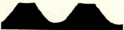
Fig. 5a—Photograph of a groove cut with a 70° feather edge stylus (i.e. a stylus having no burnishing facet). Horns of large proportions are present and substantiate the fact that grooves cut with 70° styli always have larger horns than those cut with wider angle styli (see Fig. 5b). Roughness in the groove also serves to illustrate the importance of the burnishing facet
