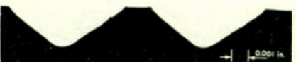
Fig. 5b—Photograph of a groove cut with a 95° feather edge stylus. A series of feather edge styli ranging from 70° (Fig. 5a) to 100° were used to establish the effect of the included angle upon the formation of horns. It was found that while none of these styli produced absolutely clean upper corners, the horns became progressively smaller as the angle was increased
