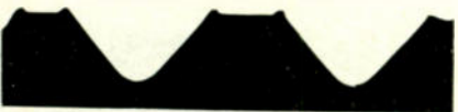
Fig. 4—"Horns" of the magnitude of those photographed were first observed in grooves cut with Master styli which maintain exact included angle specification. This led to intensive research on the subject and to the findings outlined in this article. Horns like these may be troublesome in processing. "Cold flow" which characterizes lacquer also may result in these large horns interfering with the playback stylus
