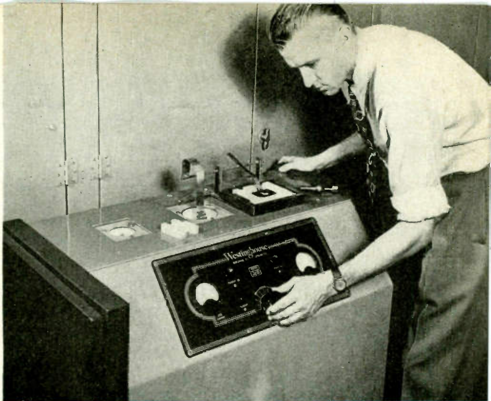
In this demonstration the 1-kw dielectric heating generator is being used to show the manner in which thermosetting glue in plywood can be made to set in 15 seconds
