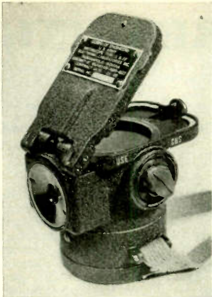
Metascope night sight produces its own power for detection of infra-red radiation
