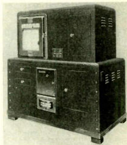
Automatic record of thermal expansion characteristics is obtained with dilatometer
