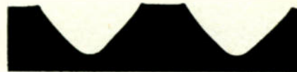
Fig. 7—Other factors being equal, the size of the horns at the corner of the groove is a function of the size of the burnishing facet. Therefore, the dimensions of the burnishing facet, at points corresponding to the upper corners of the groove, must be carefully controlled in order to keep the horns to a minimum. Changes in pitch, however, bring a different portion of the stylus into use. This may result in the width of the burnishing facet changing the upper corners of the groove. This is a photograph of deep cuts so that the narrow portion of the burnishing facet affects the corner of the groove.
