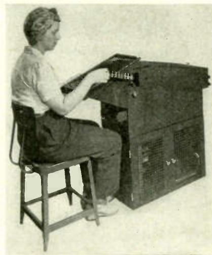
Dry batteries are fully checked by test unit
