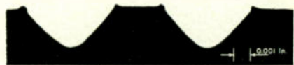
Fig. 8—Photograph of a light cut (or fine pitch) made with the same stylus used to cut the deep grooves illustrated in Fig. 7. At this finer pitch a wider portion of the burnishing facet affects the corner of the groove, producing larger horns
