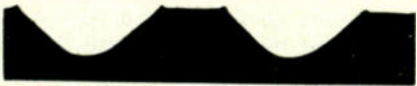
Fig. 3b—Showing the truer groove shape that is the characteristic of Master styli which are manufactured to accurate tolerances. Straight side walls and a truer bottom radius results
