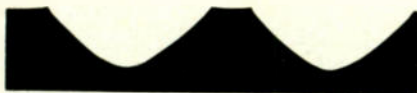
Fig. 3a—Polishing the burnishing facet around the peripheral edge of the sapphire in regular production results in some deviation from "ideal" shape. The photograph shows the recorded groove that results. The curvature of the bottom of the groove tends to follow up into the side walls, which should be straight. An increase in the included angle also occurs and a true radius is not obtained.
