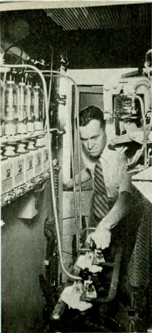
Making power level adjustments on the 20 kw 450 kc Induction heater
