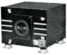
**THE 180K-1** antenna loading unit efficiently transfers the power output from the 18S-1 to any standard commercial fixed antenna. Remote controlled, pretuned operation for ten channels is provided. The nominal input impedance is 50 ohms. Weight, 10 lbs. Size,  $7\frac{1}{2}$ " h,  $10\frac{1}{2}$ " d, 12" l.
