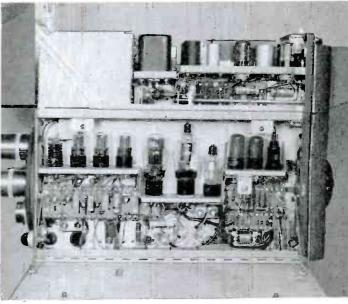
Side view of camera opened to show accessibility provided for all tubes, components and wiring. View finder cover is raised. Below are shown the separable camera and view finder sections, each an integral unit itself, removable for maintenance operations
