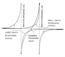
Fig. 4—Resonance curves for small, large, and combined cavities of a rising sun magnetron
