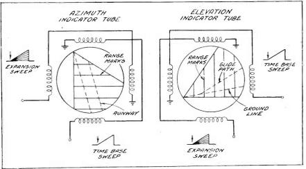
Fig. 14-Range marks are not perpendicular to runway with ordinary sweep
