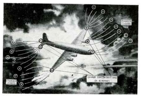
Fig. 1—Charge concentrations build up on opposite extremities when aircraft nears charged cloud
