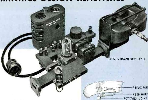
The DeMornay-Budd packaged R. F. Unit provides a complete R. F. assembly for microwave radar. It is now possible to obtain as standard items all the microwave R. F. components necessary in the fabrication of a complete radar—DeMornay-Budd Standard Transmission Line Components plus packaged R. F. Unit.
