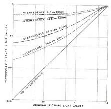
Fig. 3—Contrast reduction when dc restorer follows peak levels of sync. pulse levels
