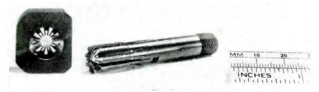
Fig. 7—1.25 cm anode with hob used to produce it. The hob is pressed into a copper blank
