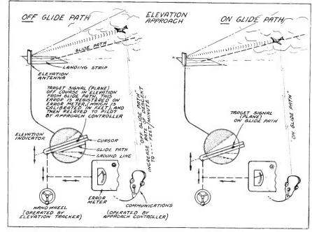
ig. 6—Error meter indication of elevation
