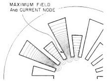
Fig. 11—Distribution of electric fields in rising sun cavities. Point of greatest field is not at mouth but inside large cavity
