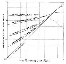
Fig. 2—Contrast reduction relations when dc restorer follows average of sync, pulse levels
