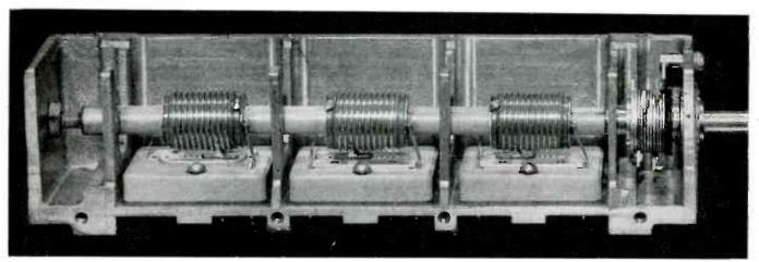
Fig. 1—Mallory-Ware inductive tuning unit which is capable of tuning the entire 13 television channels and intervening assignments to FM and other services, and which makes possible 100 to 1 amplitude discrimination against image frequency in the middle of the band
