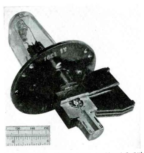
Fig. 13—A 1.25 cm magnetron with sides cut away. Note the glass window construction at end of wave-guide, the quarter wave choke grooves. Type of glass and matching are important to prevent melting
