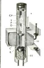
ENERGIZED—Coil C pulls plunger P down into mercury M. Mercury thus displaced enters thimble T through orifice O. Inert gas in thimble gradually escapes through ceramic plug CP.
