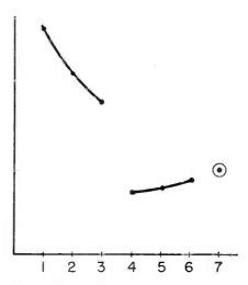
Fig. 6—Wavelength versus mode number for 14 cavity rising sun magnetron. Note the splitting of the spectrum due to alternate small and large cavities
