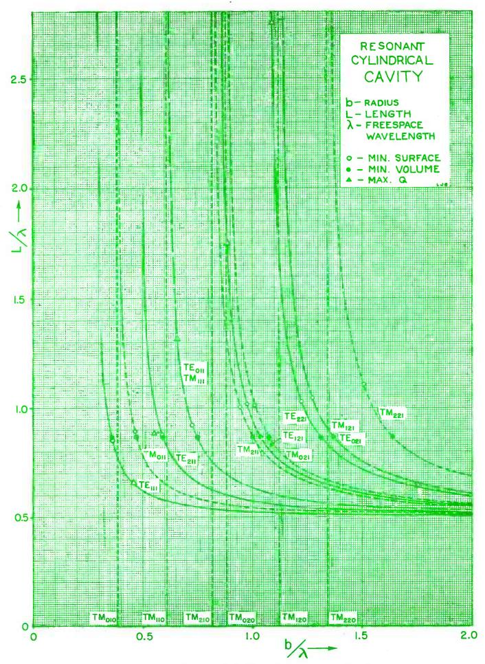
Design curves for cavities having either minimum surface or volume, or maximum Q
