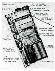
Internal arrangement of Belmont pocket radio which measures  $3 \times 3/4 \times 61/4$  in., weighs 10 oz. with batteries. It is a 5-tube superhet, tunes broadcast band
