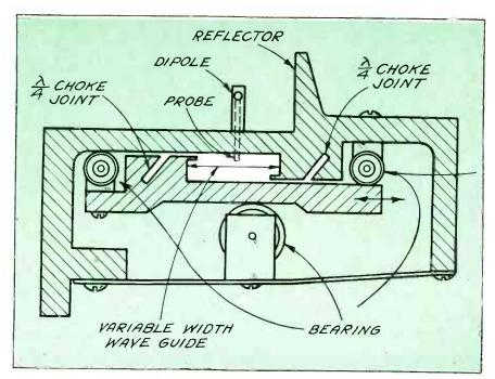
Fig. 11-Variable wave guide causes beam swings
