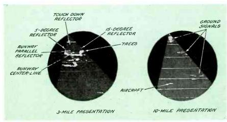
Fig. 3—Precision system azimuth indicator presentation
