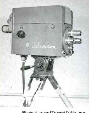
Close-up of the new RCA model TK-30A Image Orthicon camera which carries four lenses in a turret. Below, addition of telephoto
