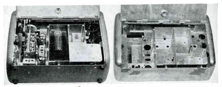
Left is a view of the new General Electric storage battery-operated portable receiver with the back cover open showing disposition of the battery, power supply and other principle components. Right is a view of the elaborate die cast foundation unit
