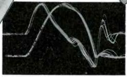
The above oscillogram revealed a flexible cam shaft which was causing faulty engine performance.
