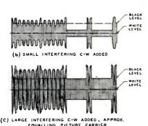
Fig. 1—Effect of interfering continuous-wave signal spaced 3 to 4 mc from picture carrier
