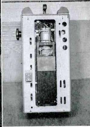
Top view of camera case with view finder section removed. All parts are accessible
