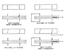
Fig. 2-Methods of mounting duplex crystals
