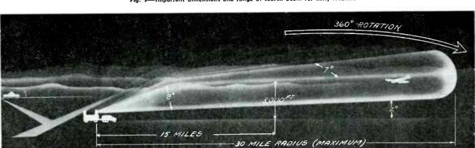
Fig. 9—Important dimensions and range of search beam for early location
