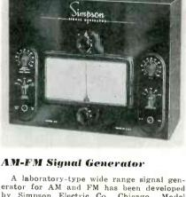
A laboratory-type wide range signal generator for AM and FM has been developed by Simpson Electric Co., Chicago. Model 415 is practically independent of line voltage variations and has constant RF output voltage throughout the frequency range. The instrument is provided with either internal 400-cycle sine wave modulation from 0 to 100% or with external modulation from below 60 cycles to over 10 kc.—Electronic Industries
