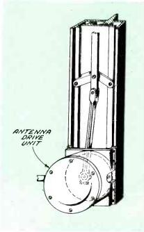
Fig. 12-Toggle wave guide mechanism
