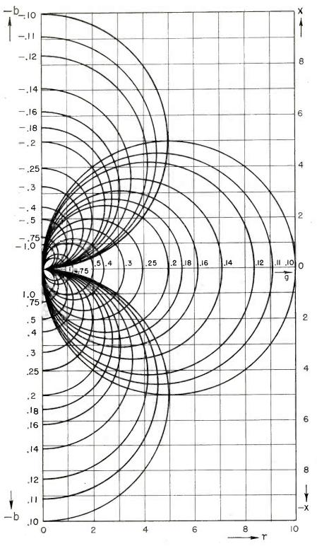
Fig. 2. Impedance-admittance chart; when  ${\bf r}$  and  ${\bf x}$  scales are divided by 10, the  ${\bf g}$  and  ${\bf b}$  scales should be multiplied by 10
