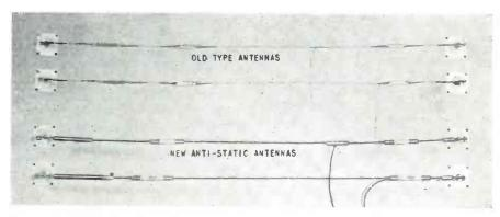
Fig. 3—At the top are shown old style open-wire antennas and below them the newer types of dielectric covered antennas equipped with anti-static hardware to eliminate noisy corona discharge
