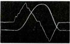
Oscillogram from same engine after cam shaft had been stiffened, showing improved performance.
