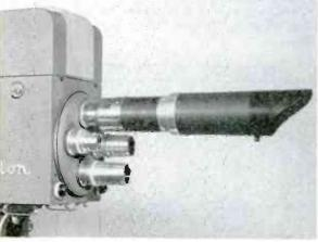
Head-on view showing arrangement of the turret lens mounting, individual lenses being positioned by rotating the turret
