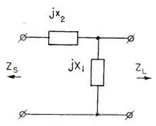
Fig. 1. Simple L-section network
