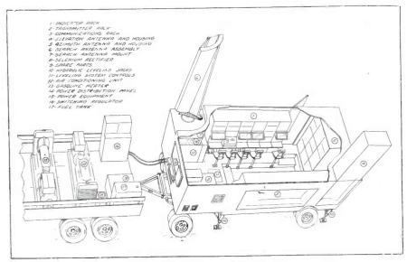
Fig. 8—Phantom view of equipment trailers showing 3 antennas
