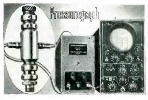
Covers wide range of engine speeds and pressures up to 10,000 p.s.i. Screws into cylinder and can be calibrated using static pressures. Vibration-proof. Accurate, dependable for frequent engine tuning. SIMPLE OPERATION — ONLY ONE CONTROL.
