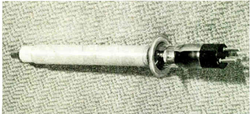
Wide range microwave oscillator tube (right) and adjustable cavity (left). Samuel and Clark (BTL)
