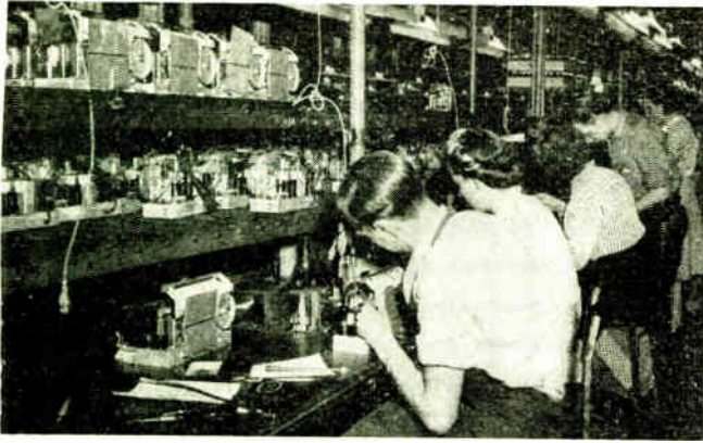
Final mechanical adjustments are made on sets delivered to and taken away from the benches by roller conveyors
