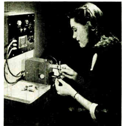
Capacitor discharge permits 60-120 welds per minute with this miniature bench type welder
