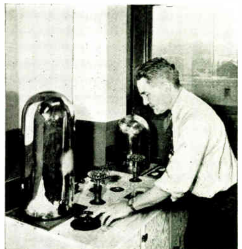
Modern pumping system for evaporating substances under test in research on Selenium Rectifiers.
