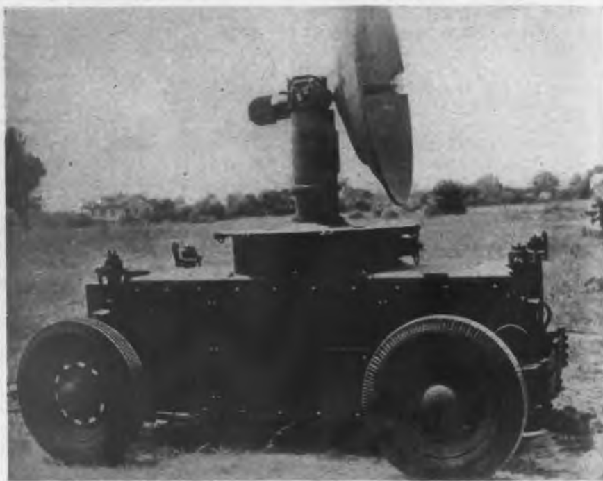
Lightweight radar equipment (AN/TPL-1) as it is rolled into operating position and below a view of the set with wheels removed and panels opened, shelter removed, ready for operation
