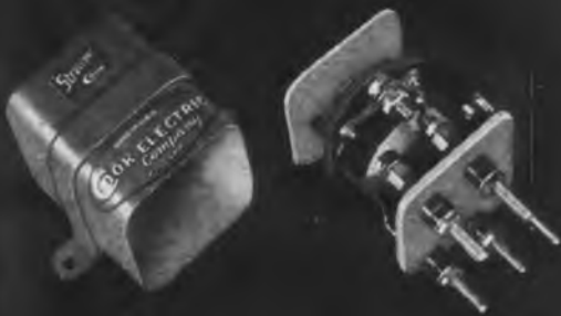
Contactors ready for Stratopaxing before covering. Wrap around mounting bracket blister on cover for adequate terminal clearance, and binding post terminals meet specifications for unit.
