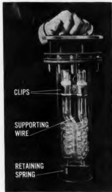
The "super" repeating flash tube built by General Electric's Lamp Department, Nela Park, Cleveland, Ohio. Arrows indicate the metal supporting parts.
