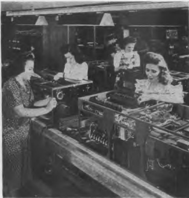
Assembly and inspection line of the step-by-step converter associated with Mark XX Radar. Below: Intricate radars designed to be slung beneath night-fighters to pin-point targets through darkness. Bomb-shaped housings enclose the radars, shown on next page, lower left
