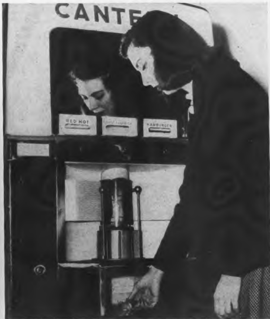
One hot dog with roll ready for the eating; and a second being cooked in the electronic oven
