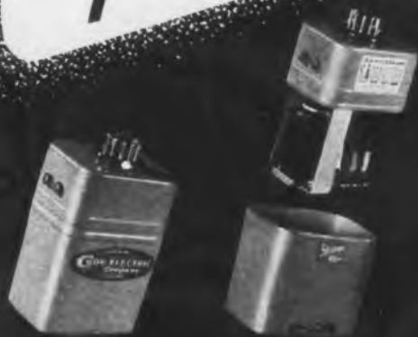
Illustration of Stratopax relay used with a machine control unit ready for plug-in connection (left) and with cover removed before gas filling and sealing (right).
