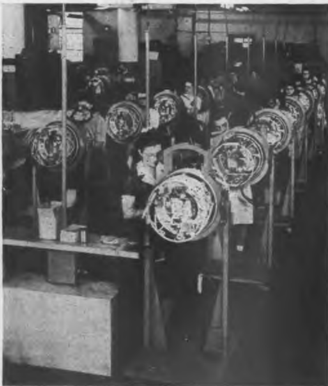
Assembly and inspection line of the step-by-step converter associated with Mark XX Radar. Below: Intricate radars designed to be slung beneath night-fighters to pin-point targets through darkness. Bomb-shaped housings enclose the radars, shown on next page, lower left
