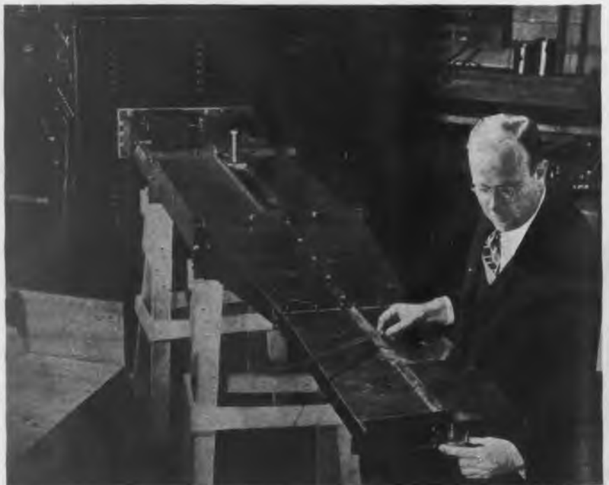
To focus electronic heat on restricted areas for many industrial jobs, Westinghouse is developing a new dielectric heating unit which projects high frequency heat at work. This method shows promise in eliminating scorching or burning in work consisting of irregularly shaped forms
