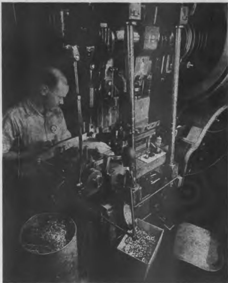
Above, automatic feed punch presses turn out a stream of accurately-dimensioned metal parts for RCA tubes. Below, an Acorn bulb machine. Glass in cane shape is fed into rack at top and is cut and formed into the half shells used in Acorn tubes
