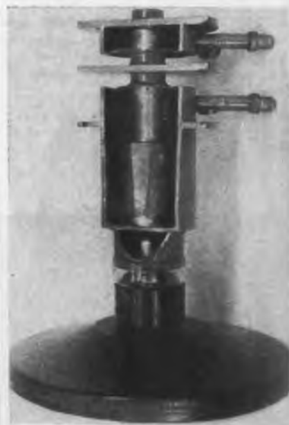
Cutaway view of Klystrons, multiplier above, triple cavity amplifier below
