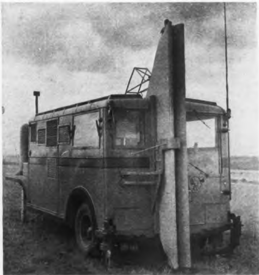
View of rear of glide path trailer showing half-cheese antenna fed by wave guides
