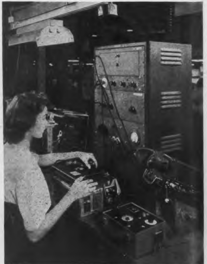
Testing the test equipment; a signal generator receives final operation test before going into the field to check radar performance. A radar is no better than its associated test equipment. When no target appears on the screen, either no target is within range or the electronic equipment is not functioning properly. Test sets tell tale.
