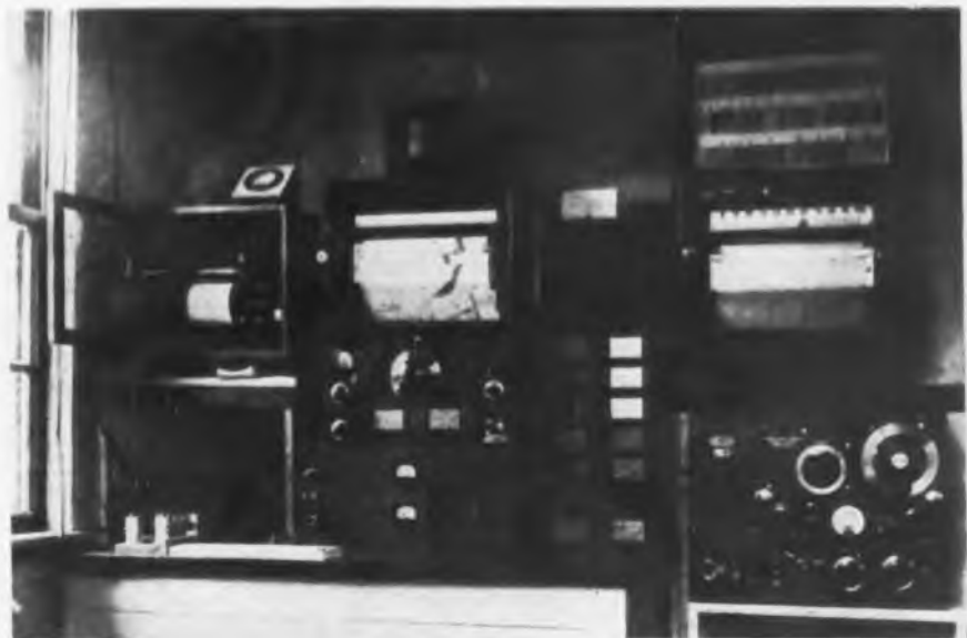
One of the field intensity recording equipments at the Cosmic Terrestrial Research Laboratory of the Massachusetts Institute of Technology—used in making the measurements recorded above
