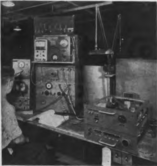
Radar elements which helped to aim big guns that mowed 'em down. With high precision test set, expert radar technician makes final tests of fire control radar prior to installation aboard a U. S. battlegewagon
