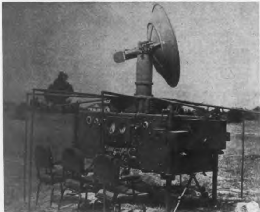
Lightweight radar equipment (AN/TPL-1) as it is rolled into operating position and below a view of the set with wheels removed and panels opened, shelter removed, ready for operation
