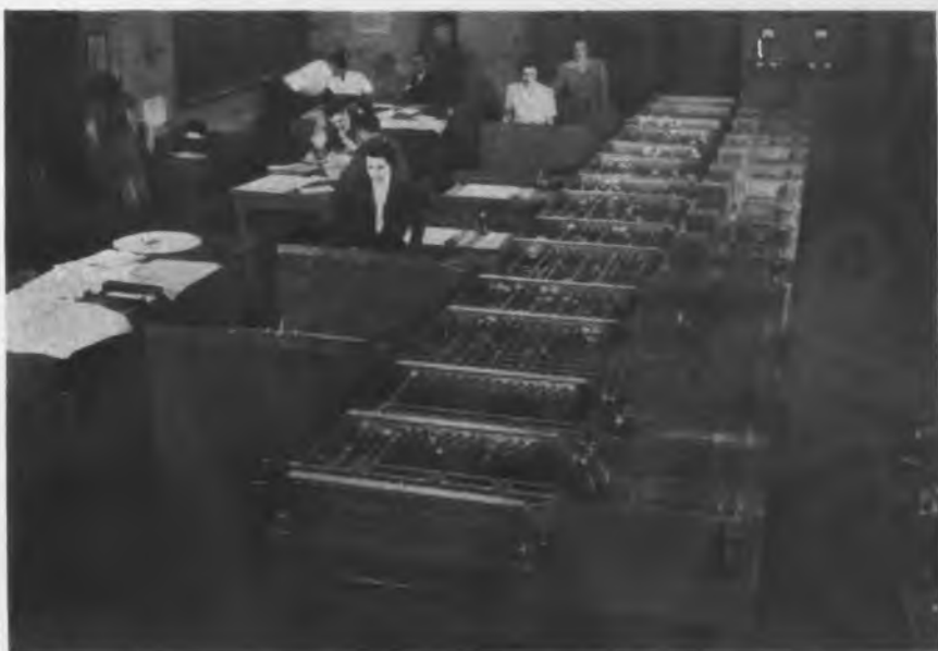
Highly sensitive polaroid photoelectric systems in this mechanical brain will permit the handling of differential equations with fourteen simultaneous integrations.
