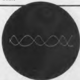
Comparison of input and output of phase inverter. Distortion in phase inverter is evident.
