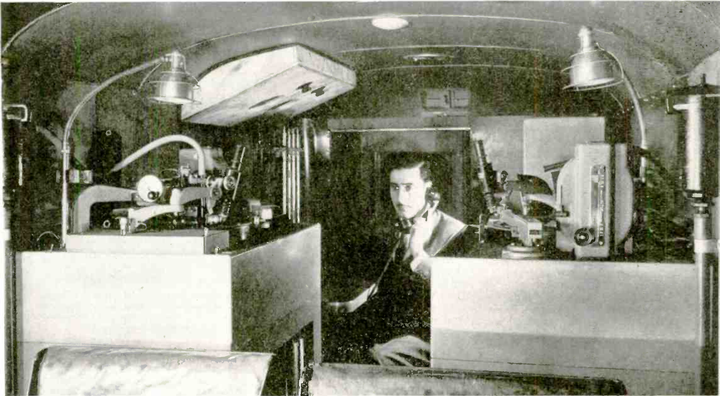
This close-up view was made through the windshield and shows arrangement of the two RCA recording lathes, with the operator in normal position seated at the console controls. Right, below, is a view showing the insulated well holding the 1 kw motor-generator set
