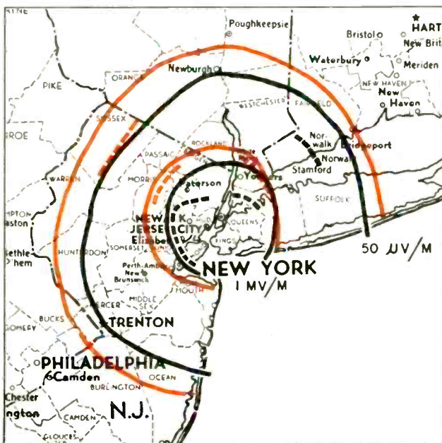
Fig. 4—Contour map showing calculated and measured field strengths for old antenna, and in red, for the new
