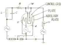
tor 14 and will cause it to be less negative; plate current will decrease to a minimum. The tube will then discharge the electric charge on capacitor C and another cycle will start.
