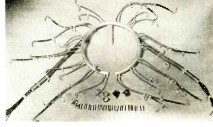
Complex ignition shielding harness required on radial type military aircraft engine. Such harness must of necessity have many joints in the conduit, to facilitate assembly and repair
