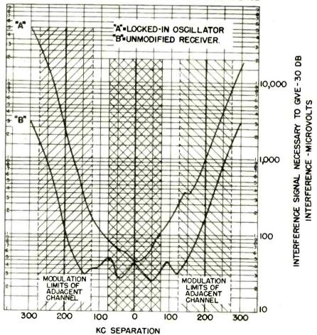
This chart, comparing signals received on an unmodified FM receiver and on one of the new type super FM circuits shows the greatly improved, single peak selectivity given by the latter
