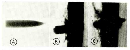
Fig. 4—High speed X-ray picture of bullet piercing armor plate. (A) Stationary X-ray picture of cal. .30 armor piercing bullet. (B) High speed X-ray picture of this bullet penetrating  $\frac{1}{2}$  in. thick armor. (C) High speed X-ray picture of same bullet 20 millionths of a second later
