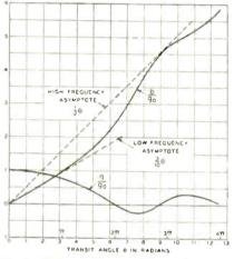
Fig. 3—Diode admittance with complete space charge
