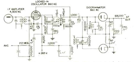
Fig. 2—The local oscillator is locked-in with and modulated by the received signal at onefifth the intermediate frequency. The discriminator is designed for the reduced frequency
