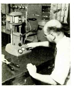
Mounting a specimen of iron powder in a suitable resin for subsequent examination
