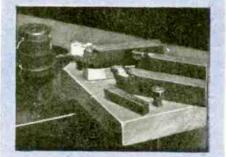
Carbide tool tips are brazed to shanks with better bond by high frequency heating.
