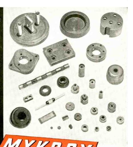
HE perfection of MYKROY #51, glassbonded mica ceramic insulation, which can be injection molded, and the processes developed for handling it rapidly and uniformly has opened a new field of applications. It is now possible to produce injection molded plastic ceramic parts of MYKROY having shrinkage characteristics of less than .001" per inch. In addition, parts molded from MYKROY #51 can be machined by grinding, drilling, tapping or cutting.
