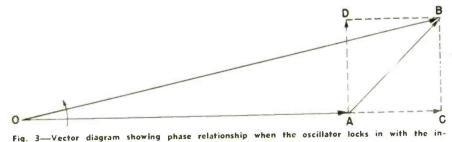
Fig. 3—Vector diagram showing phase relationship when the oscillator locks in with the incoming signal; vector AB then makes a constant angle CAB with OA
