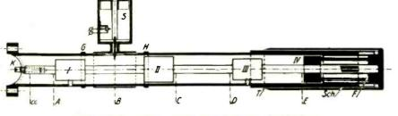
Wavemeter for 140 mm. waves detects changes of 0.0007 mm.
