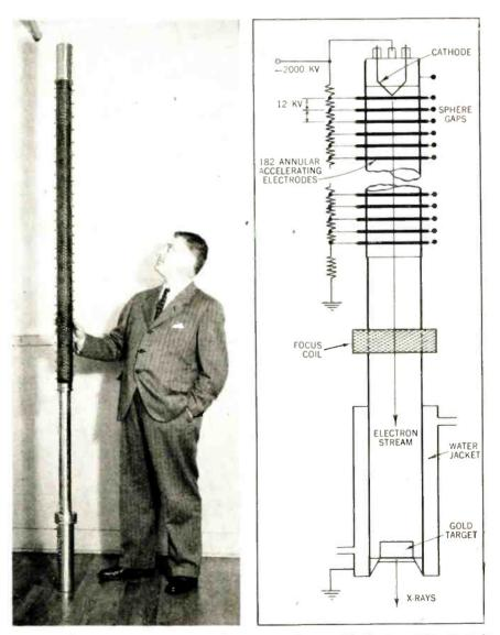
At left, R. R. Machlett, president of Machlett Labs., holds new 2000 kv X-ray tube. Cathode end is at top and water jacketed target at bottom. At right is outline of accelerating column, focus coil, target and water jacket. X-rays are transmitted directly through target
