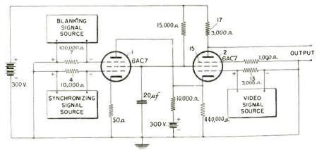
cut-off region where the space current is practically independent of grid voltage variations. The current through tube 2 will be further reduced by the synchronizing signal.
