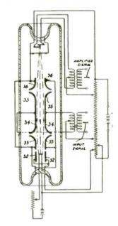
the plates as shown in the drawing. The adjacent portions of each pair of plates 33, 34 and 35, 36, respectively, are flared outwardly; an abrupt flare is required. F. Gray, Bell Telephone Laboratories, (F) May 31, 1941, (I) June 13, 1944, No. 2,351,501.
