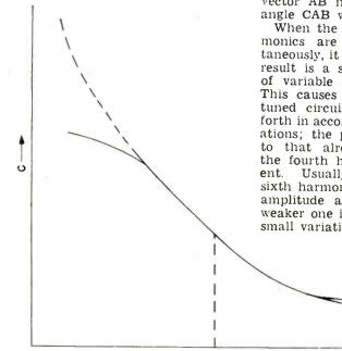
Fig. 4—Solid line is falling input capacitance of discriminator; dashed line is variation of capacitance needed to keep the oscillator in tune as the frequency is varied
