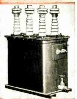
300 VA Filament transformer, single phase, 60 cycles, 6 secondary windings of 5 volts each; 3 secondary windings operating 40 KV above ground and 3 secondaries operating 20 KV above ground.
