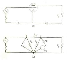
Fig. 1—Conventional representation of vacuum tube network
