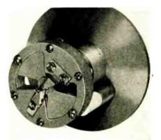
stator sections. These devices can be designed with a wide variety of characteristics, and with tuning ranges as high as 12:1 and with Q values of 300-650. Another form of tuning arrangement found of value is the cylindrical circuit also shown. A special shaped split cylinder rotates inside to produce the tuning variations.
