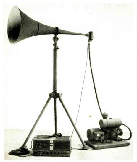
Portable units are operated by either electric or gas engine drives. Fig. 4 shows a form of the latter, with source of power for amplifier and air compressor mounted integrally on the gasoline engine base, Fig. 5
