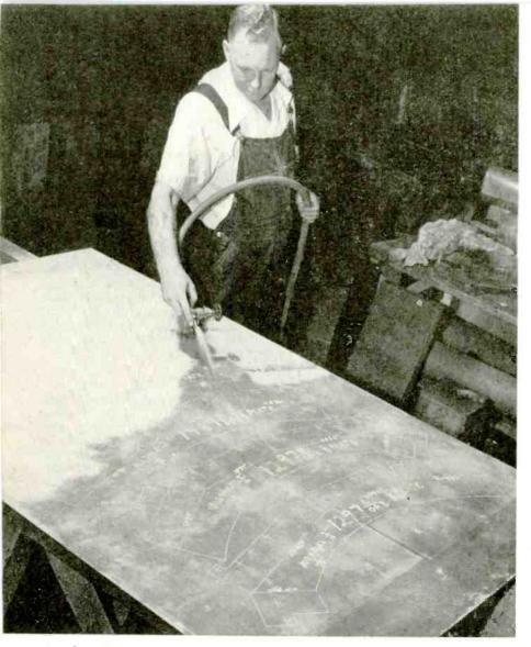
I —Ilat metal work is speeded up by Eastman Kodak Co., Rochester, N. Y. Kodak Layout Paint is sprayed on. Black ink drawing is photo-printed on metal by exposure to arc or mercury vapor lights. Print is "developed" by warm, weak, ammonia water and washed
