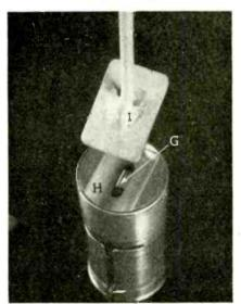
denser is discharged across such a tube, a cathode hot spot is formed, and the space charge being relieved by the positive mercury ions, heavy currents will flow.
