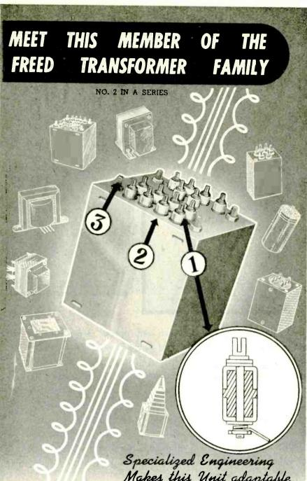
1. A cross-section of the husbing assembly, showing special neoprene gasket which insmess perfect her-metic sealing and is completely fungus resistant. Sturdity con-structed screw machine part set in high dielectric steatile busbing makes wiring and soldering easy.
