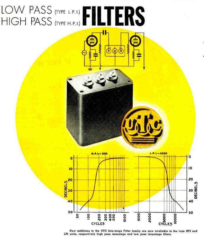
The units are designed with a nominal impedance of 10,000 ohms to be used in a circuit as illustrated. Typical curves obtainable are shown above. Loss at cutoff frequency is less than 6 DB. At .75 times cutoff or 1.5 cutoff frequency respectively, the attenuation is 35 DB, and at one-half or twice cutoff frequency respectively, the attenuation is 40 DB.
