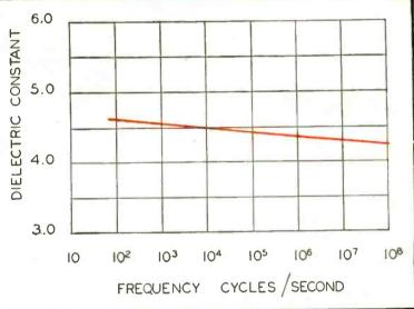
These data represent average values measured at normal laboratory conditions of temperature and humidity on specimens not previously conditioned.
