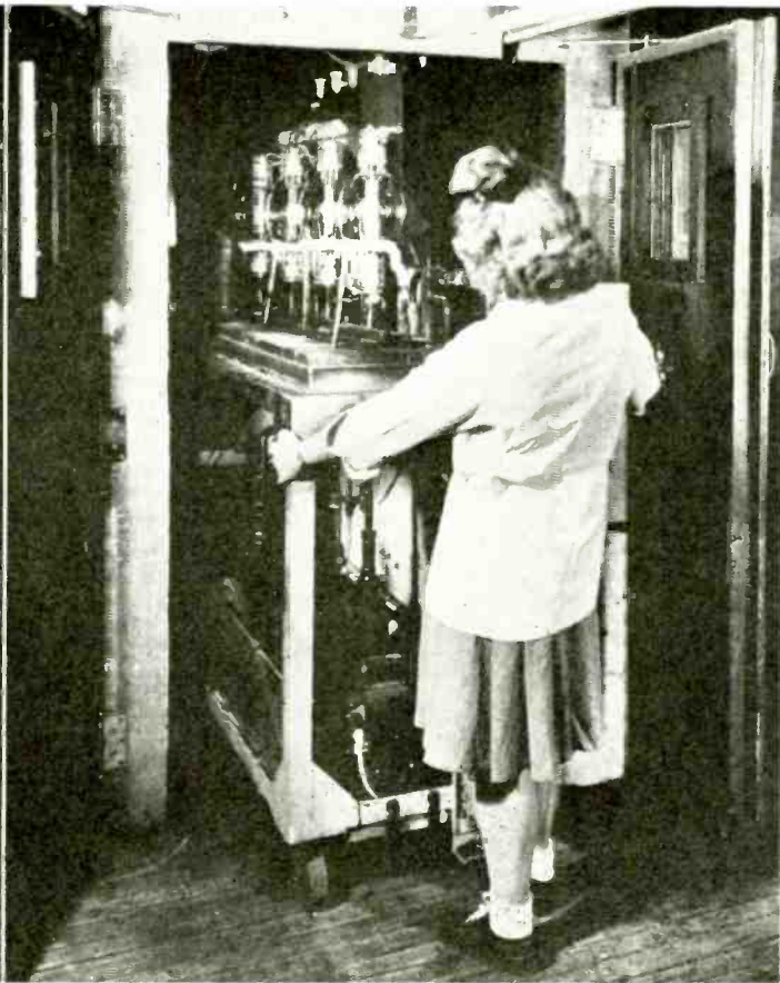
5—Upon completion of high voltage processing which can be inspected through lead glass, dolly is removed and tubes are sealed off
