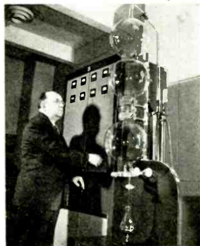
Dr. George Brown, of RCA Labs, with demonstration model of his high freq. penicillin drier
