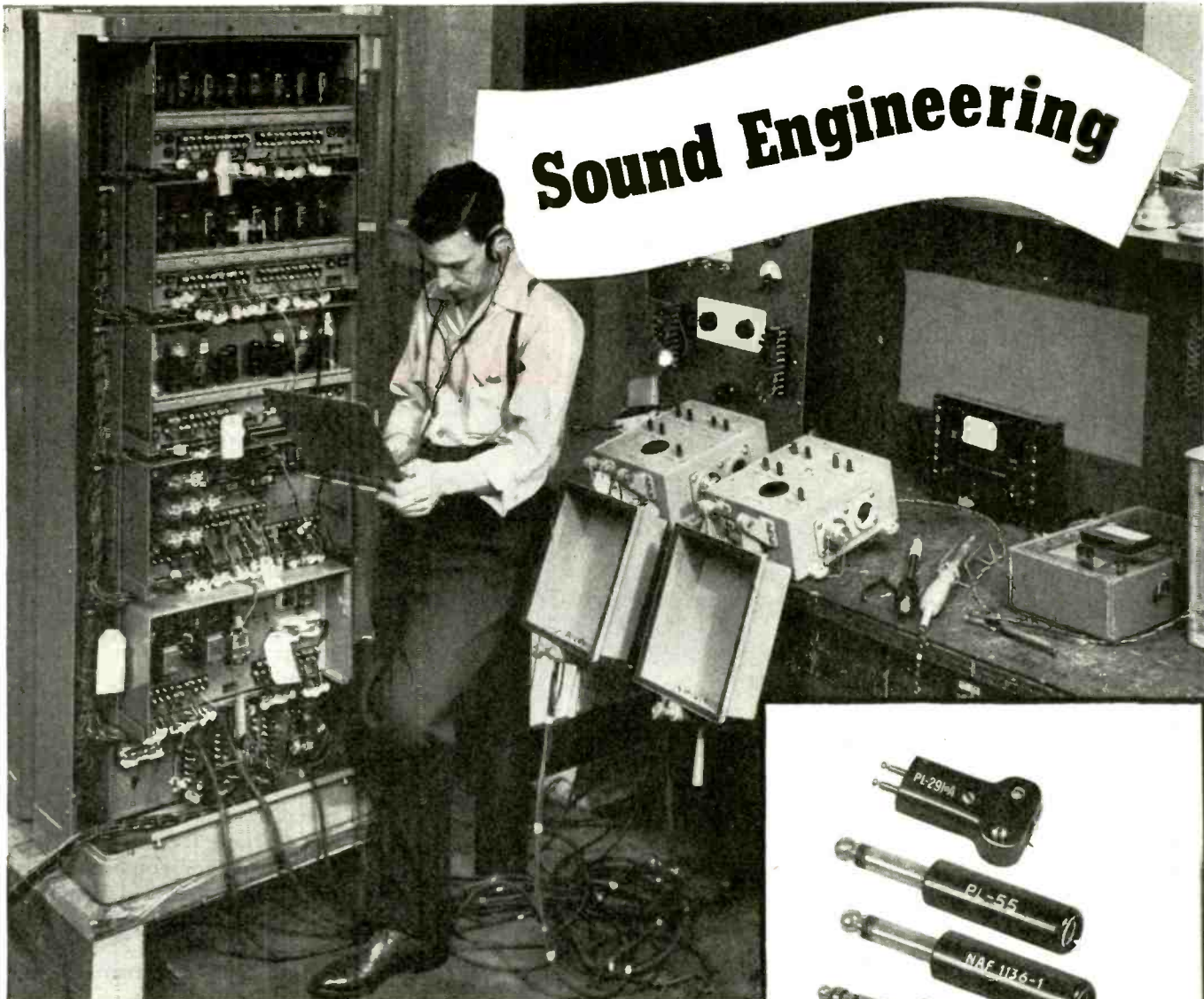
Final test—Remler marine amplified sound transmitting equipment.
