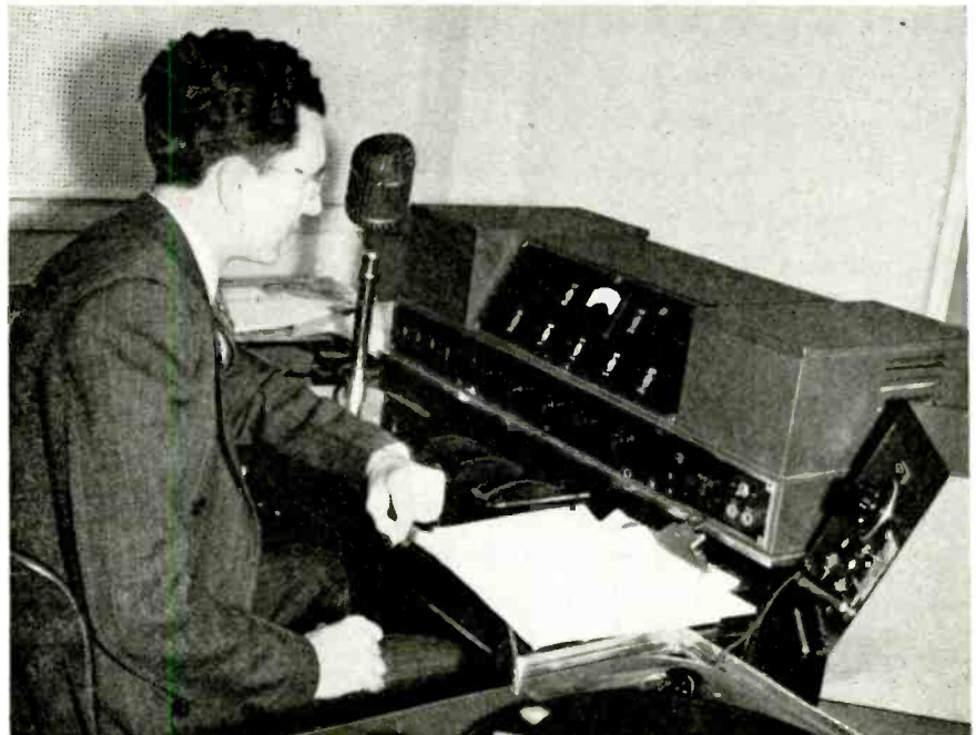
Standard type Western Electric model 23C broadcast studio console
