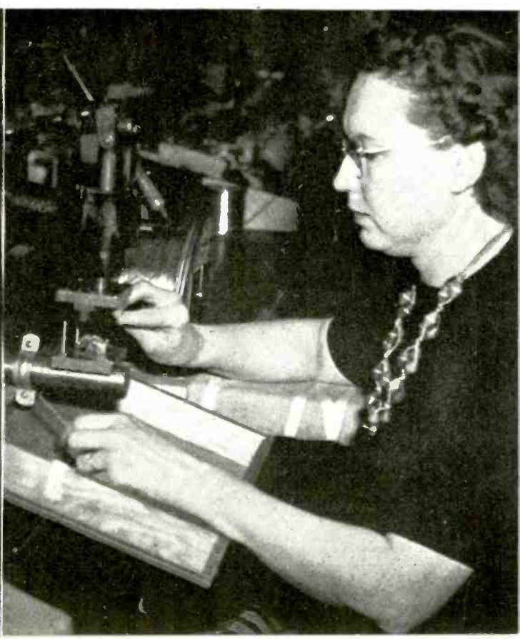
9 Two operations formerly separately performed can frequently be combined into one, at great savings of man and machine time. Photo shows $50 bond winner at Farnsworth Television and Radio Corporation's Marion, Indiana, plant. Girl operator demonstrates special punch and die set to form and cut wire in a single operation
