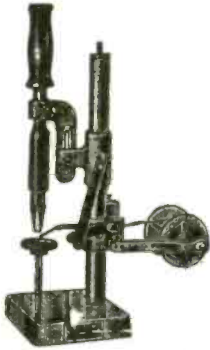
SPOT SOLDERING MACHINE designed for treadle operation for advancement of iron and solder, leaving operator's hands free for handling of product.
