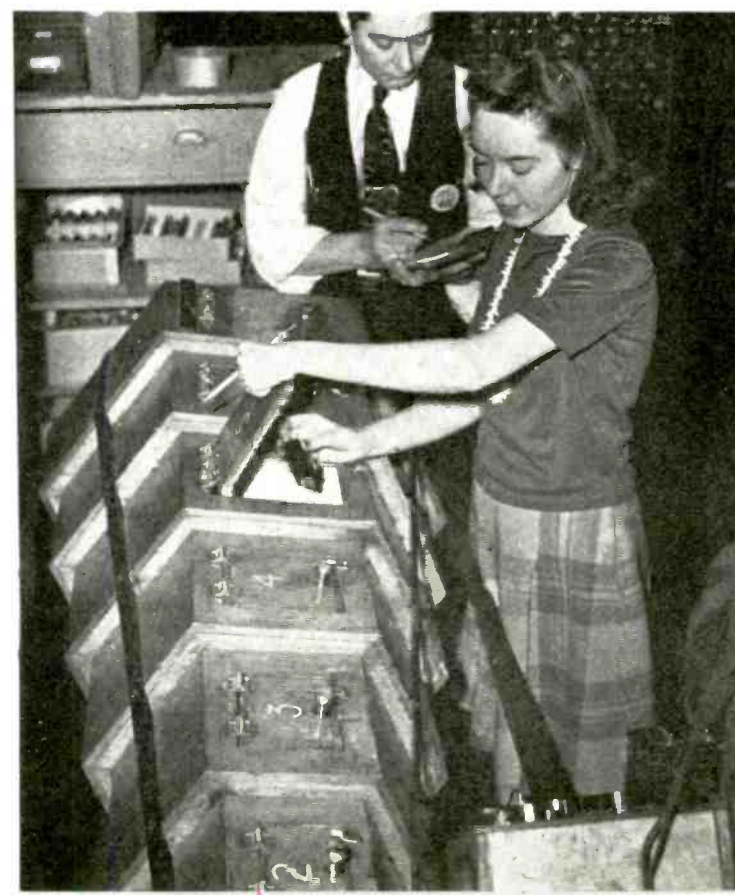
8 Rotary drop test unit at Tung Sol, Newark, N. J., is useful research tool and production quality test instrument. Graduated hexagonal boxes rotate on common shaft. If normal breakdown of a certain tube type occurs in Drum No. 5, it is henceforth known as "bogie drum" for that type. All production must then pass tests up to No. 6
