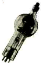
PHANOTRON — for high-frequency electronic heating
