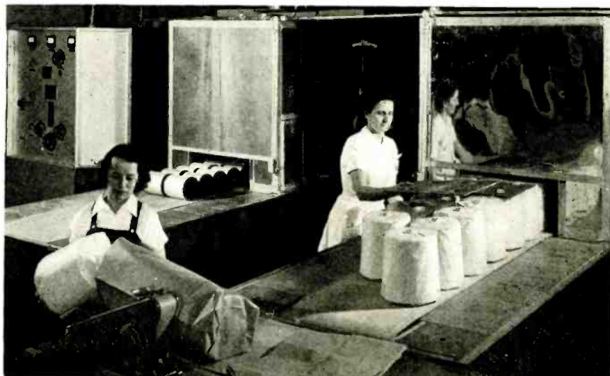
Electronic heating introduces new process of textile twist-setting at Industrial Rayon Corp.
