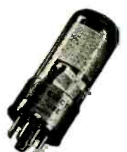
PENTODE — a general-purpose amplifier
