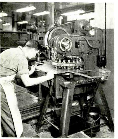
PUNCHING 100 HOLES in radio chassis needed in small lots at Federal Telephone and Radio Corp., Newark, N. J., with turret-head punch press designed for short run piercing operations
