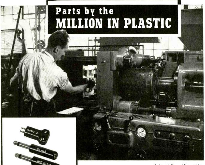
Remler injection molding machine. Other complete facilities to handle every type of plastic molding.
