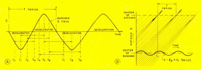
Effect of buncher field on electron velocity at A and Applegate diagram of bunching at B. Slope represents velocities
