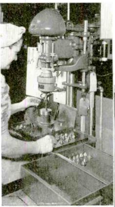
AIR OPERATED CHUCK speeds precision work on small round parts and largely does away with need for special jies and fixtures. Tappling operation illustrated. Air chucks, made by Redmer Air Devices Corp., Chicago, give collet capacity up to one and three-fourths inches
