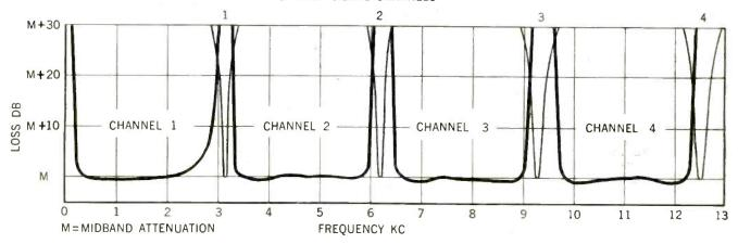
Relative overall transmission frequency characteristics of four-channel tadio carrier telephone system. Channel bandwidths are representative of overall audio transmission characteristics measured between two-wire terminations
