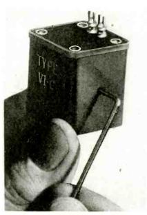
use in oscillators, (a model with 30 per cent tap for Hartley circuits is available), tuned amplifiers, equalizers and filters. It is housed in a die cast case, weighs approximately 5 oz. and the inductance is varied by means of an Allen wrench. There are nineteen standard types, from .0085 to 33.0 henries.
