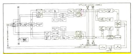
Block diagram of direct line and No. 2 carrier channel as applied to wire lines. Frequencies of filters and oscillators in other channels are shown on the chart below, which illustrates assignments for several typical systems
