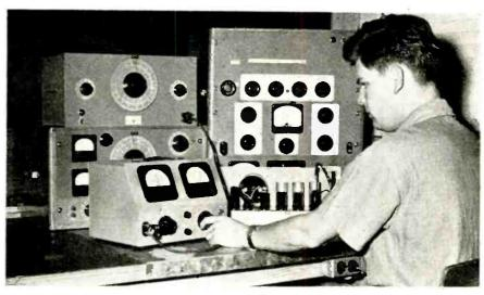
General view of the low frequency voltmeter (instrument with sloping panel) in use for the measurement of the low frequency characteristics of an amplifier
