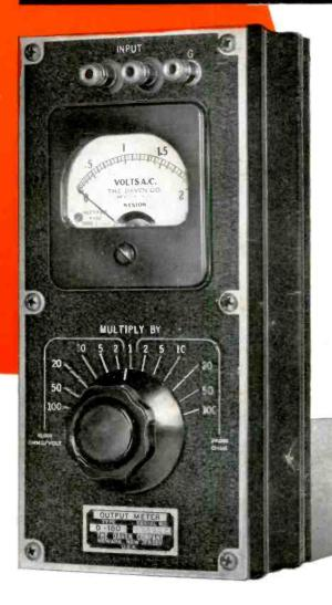
The DAVEN D-180 Output Meter is a combination of a high impedance voltmeter and a constant impedance output meter. The high impedance voltmeter range is particularly convenient when measuring transformer secondary voltages and as a bridging indicator where a high impedance is required. The constant impedance range serves as a null detector and as a beat indicator in the comparison of two frequencies.
