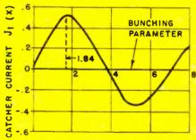
Fig. 6. (Above)—Variation of rf catcher cure rent for bunching parameter X as given by equation 3
