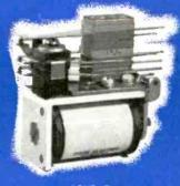
ABOYE—Type 108—Antenna switching contact combination with Mycalex insulation. Has a side contact mount to reduce capacity between antenna circuit and ground.
