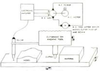
Tube-controlled tracer mechanism for intricate surface-machining
