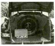
Method of mounting the FM transmitter in one of the California Highway Patrol cars
