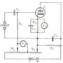
Fig. 1—Schematic showing the components in the vacuum tube voltmeter for low frequencies
