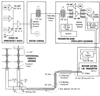
Photograph above shows arrangement of the  $\frac{1}{6}$ -in. coaxial line, the  $\frac{1}{4}$ -wave balancing transformer, the  $\frac{1}{4}$ -wave matching transformer, and start of the 250-ohm line shown schematically
