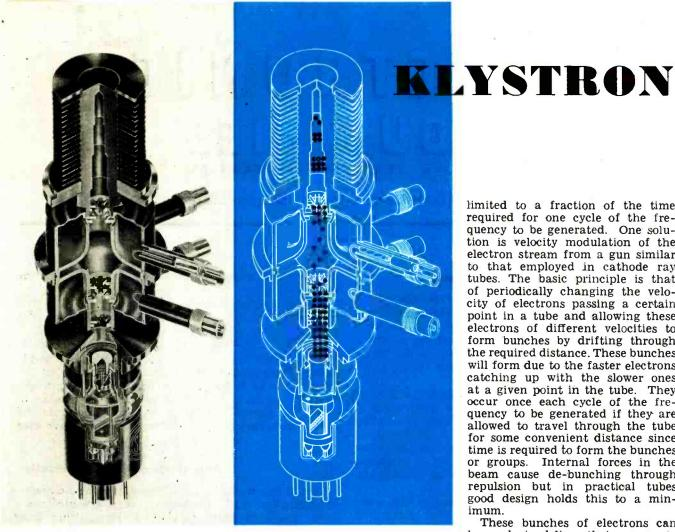
Fig. 1-Sectional view of 410R showing electron gun at bottom, lower (buncher) cavity, upper (catcher) cavity; pickup loops with seals, and heat radiating collector at top. At right, buncher action is shown altering electron velocity. Groups form at catcher and deliver energy
