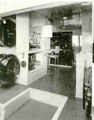
Cable reels, provided with brakes, are at the left rear with motor generator and B battery compartment just ahead
