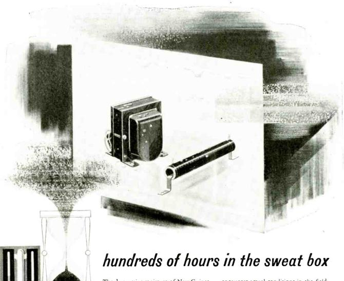
The destructive moisture of New Guinea jungles or a London fog is duplicated in this high humidity chamber in the Utah laboratory.
