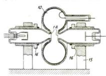
this type of tube from a glass pipe is extremely simple. To tune the resonator, pressure is exerted by turning screw 16 so that the two openings 12 come closer together. The glass yields sufficiently to permit tuning of the circuit within limits. Several resonant chambers may be blown consecutively in the same glass pipe. E. Steudel, General Electric Co., (F) Aug. 30, 1941, (I) March 7, 1944, No. 2,343,487.
