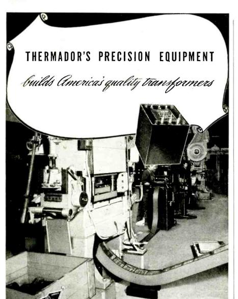
Two of Thermador's automatic high speed lamination presses
