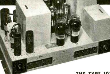
Imput impedance 600 ohms and bridging. Gain 600 ohm input 61 db., bridging input 46 db. Frequency response 30 to 16,000 c.p.s. either input—600 ohm output ±.5 db., 30 ohm output ±1 db. Power output—production run average: +47 V.U. with less than 3% RMS harmonic content.
