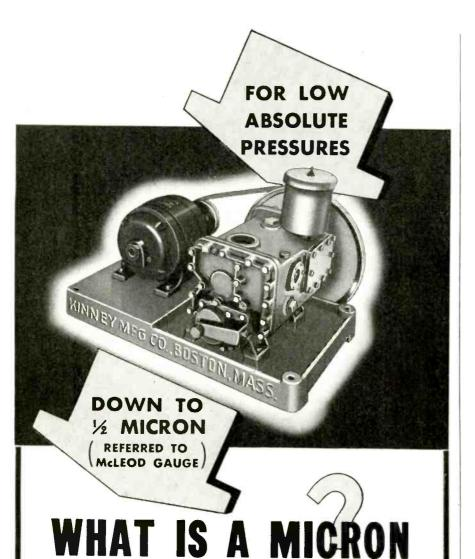
Has it legs? Does it bark like a dog? Many people using vacuum pumps and working with microns couldn't identify a micron if they saw one. When used in reference to pressure (absolute) a micron is the weight of a column of mercury 0.001 millimeter in height. A column of mercury 1 MICRON (.001 mm) in height produces a pressure in pounds per square inch of 0.0000193, which is mighty close to nothing. But every KINNEY Compound Dry Vacuum Pump must pump down to 0.2 micron before being shipped!
