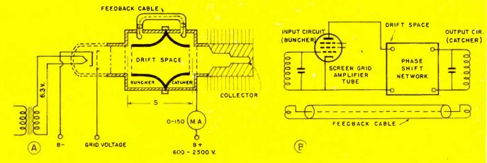
Fig. 7. Klystron tube at A showing bunching distance 5 and equivalent conventional tube circuit at 8. Phase-shift network replaces drift space
