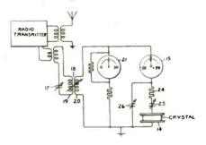
which the crystal may be used, variable capacitor 25 is inserted; the resonant frequencies of the quartz, and consequently the useful frequency range, is lowered when its capacitance is increased. The sensitivity of the device, or the slope of the impedance-frequency curve within the useful range, may be regulated by varying capacitor 26; an increase in capacitance will cause an increase in sensitivity. C. F. Baldwin, General Electric Co., (F) Oct. 7, 1941, (I) March 7, 1944, No. 2,343,633.
