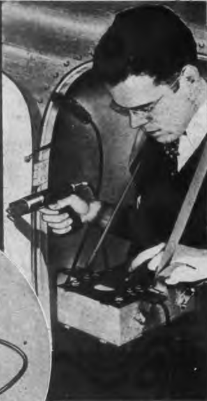
The modern way to test bond or contact resistance down to 0.0001 ohm.
