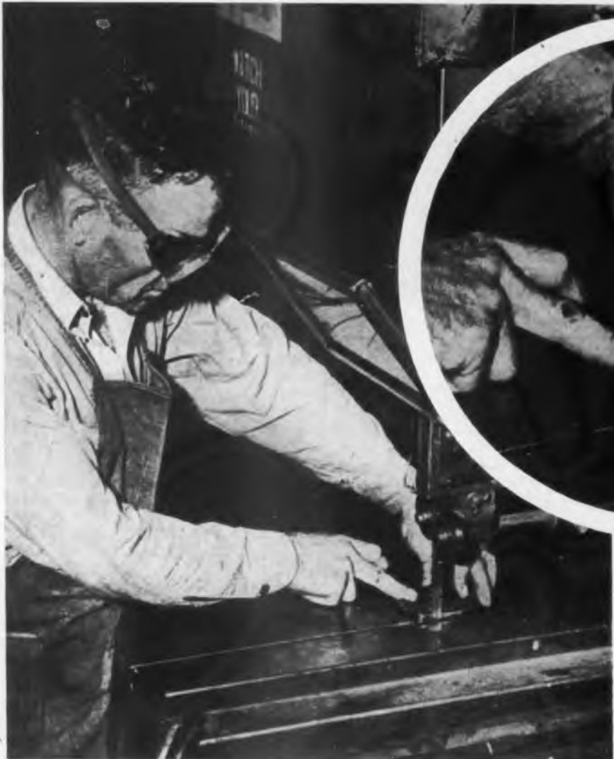
1. ↑ FIXTURES or templates used with band saw at Yellow Truck and Coach Co., Pontiac, Mich., speeded up production by eliminating time-consuming marking-out operations formerly required
