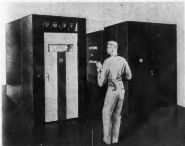
Fig. 8—100-kw radio frequency oscillator operating at 25 megacycles for production of heat to dry rayon
