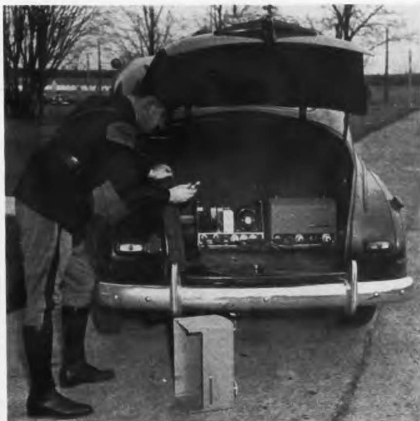
The 50-watt mobile FM transmitter, and the receiver, are mounted on wooden base boards which are floated on rubber on brackets welded to the car frame
