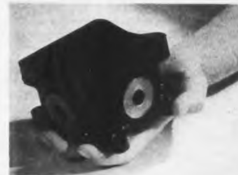
Top—Pre-forms of raw plastic before heating. Center: Electrodes with pre-forms in position. Bottom: Finished plastic outlet box as it comes from mold
