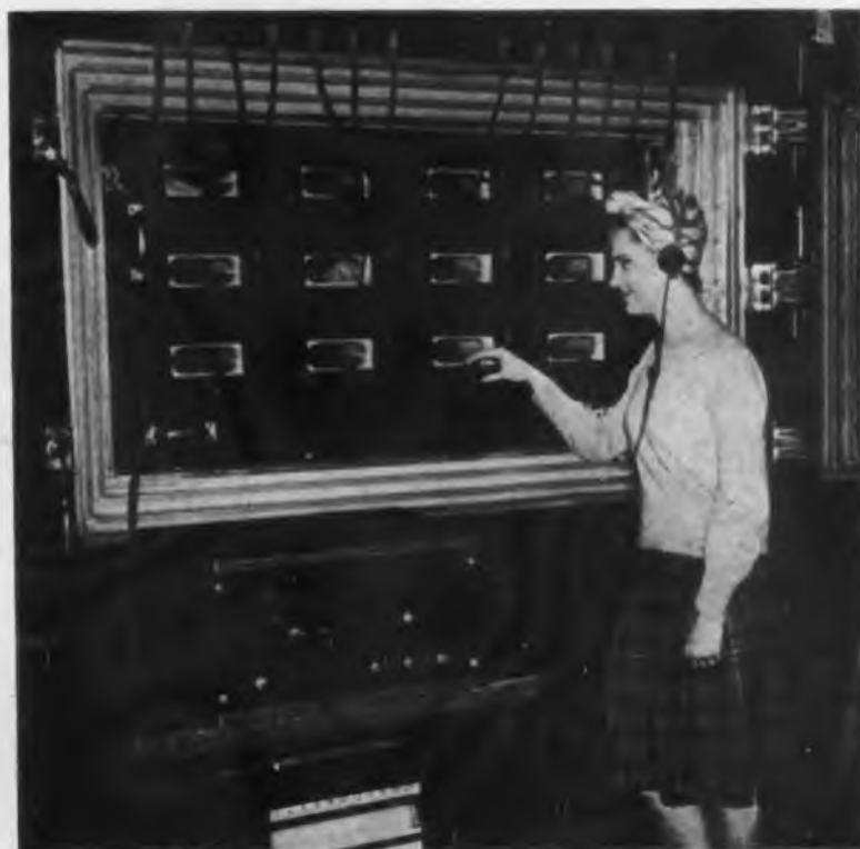
Fig. 1—Temperature compartment (American Collis) equipped with facilities for checking frequency drift of 12 Cardwell frequency meters, mounted behind windows in auxiliary panel of refrigerator. Frequency converter and Celecgray recorder on rolling wagon. Buffer and control tubes mounted above door with removable leads disconnected when main door is closed
