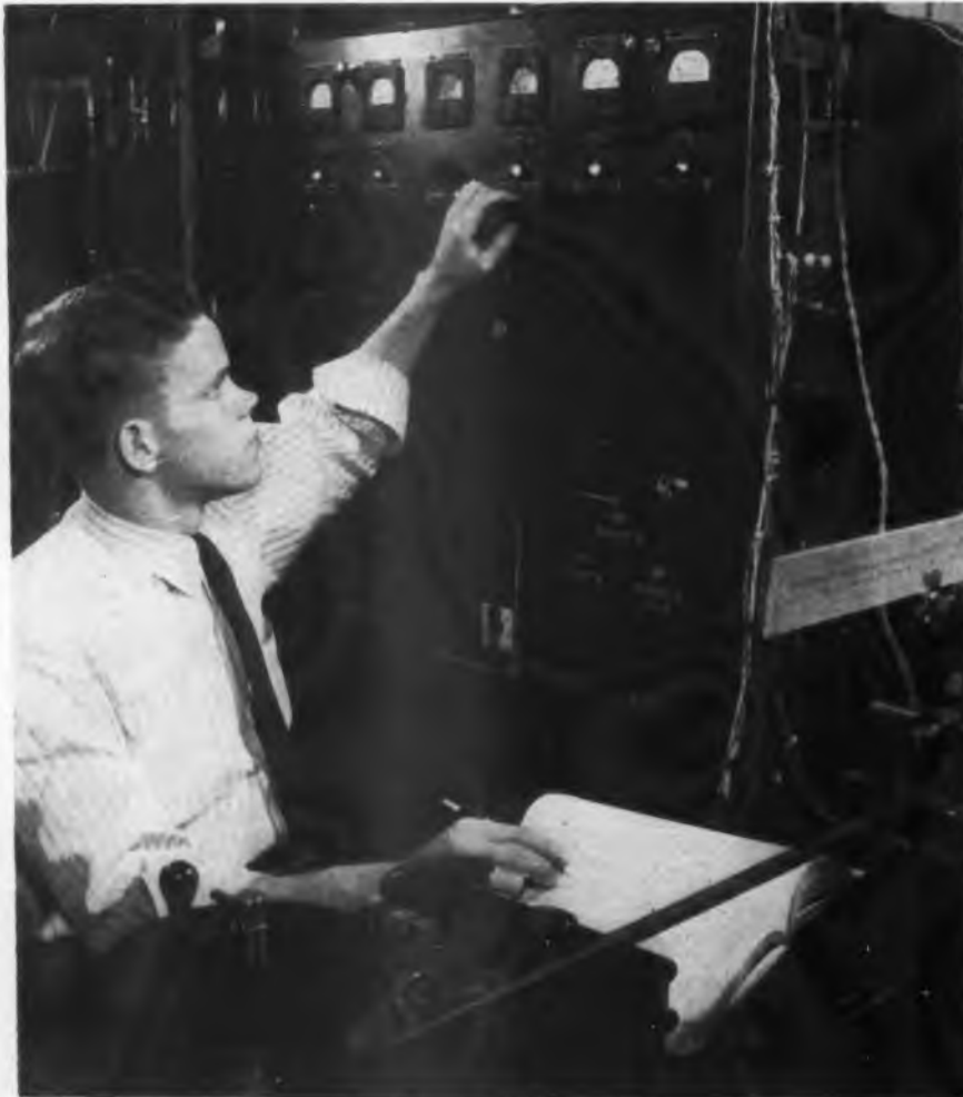
Ready for work in refinery or chemical plant, the latest model of the mass spectrometer uses 15 kw at 110 volts. Cuts time element considerably
