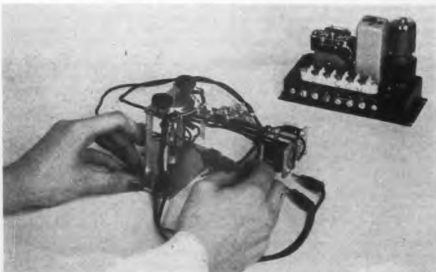
2. ↓ ASSEMBLY TIME of electronic pyrometer controller cut down by employing Bristo multiple spline socket screws instead of tiny hard-to-hold slotted-head screws
