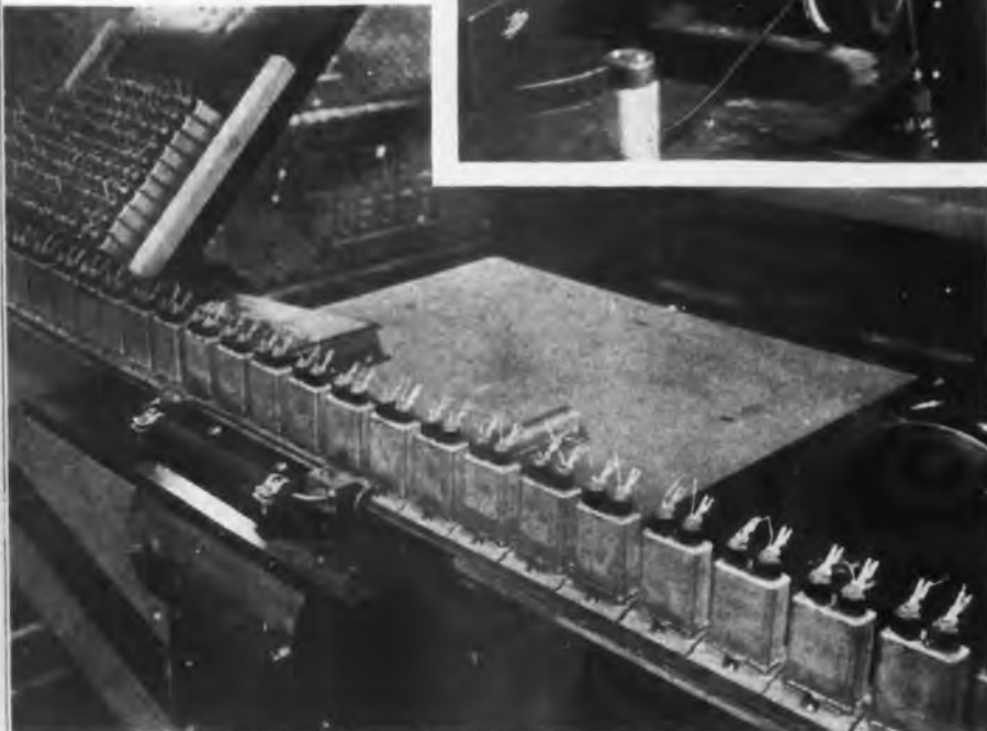
Fig. 4—Soldering of bases on capacitor cans has been stepped up from 100 to 2500 an hour at RCA Victor through application of rf induction heating
