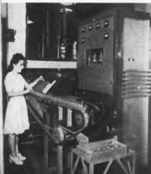
Fig. 1—Continuous soldering set-up for sealing capacitor containers
