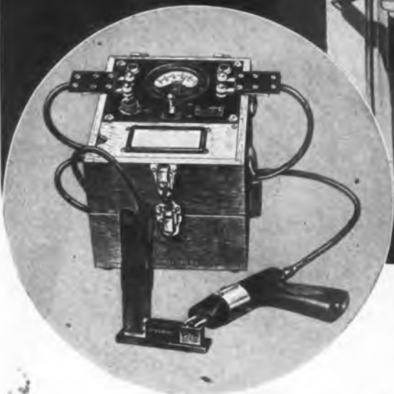
The modern way to test bond or contact resistance down to 0.0001 ohm.
