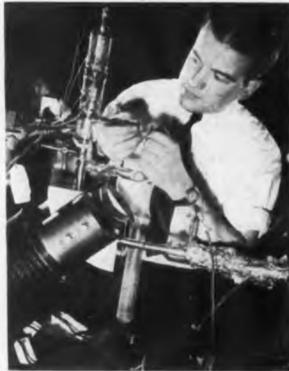
Curved tube passes between two poles of electromagnet of mass spectrometer
