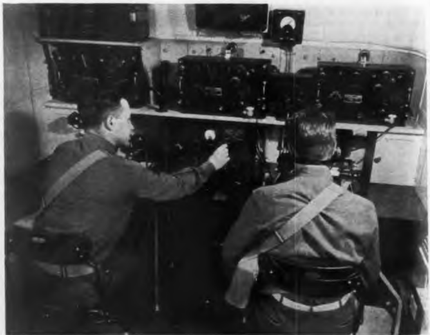
Modern mobile Signal Corps message center, showing kind and extent of radio transmitting and receiving equipment installed in a large trailer and used to maintain constant communication between ground units and supporting air cover
