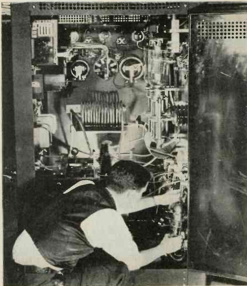
General view showing internal arrangement of the 15 kw heating equipment with the operator inserting one of the rectifier tubes
