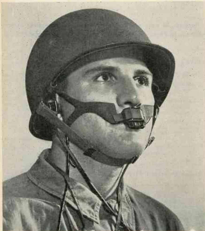
Soldier equipped with lip mike and hearing-aid type earphones
