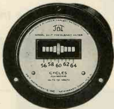
Size- \frac{3}{4} " flange, dull black metal case for flush panel mounting, 9 or 11 reeds, full or half cycle increment. Reed in resonance vibrates as shown. Simply READ THE REED, and that's your frequency.
