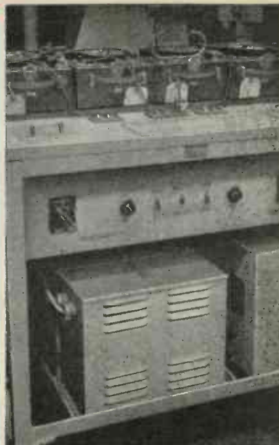
EXTREMELY CLOSE VOLTAGE REGULATION , so essential to speedy, accurate production-line testing, is automatically maintained by a 500-volt-ampere G-E stabilizer on a test bench in a fluorescent-ballast factory.
