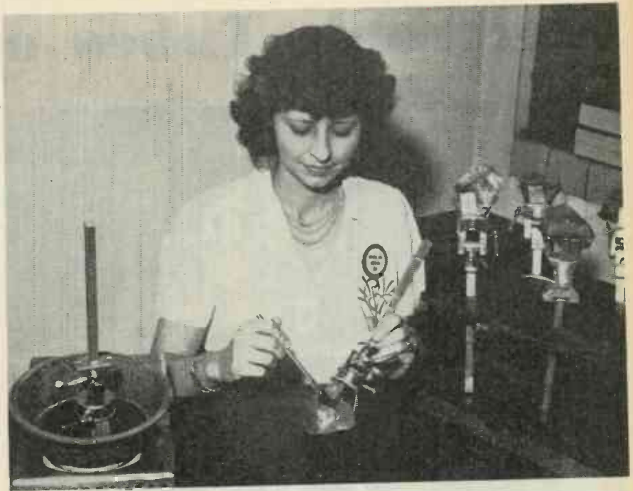
Heated crystal is cemented to three-prong holder with adjustable positioning head
