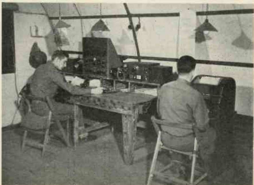
The Army's new long wave receiving stations in Arctic Circle areas look like this. Transmitters are located elsewhere and remote controlled through keying lines
