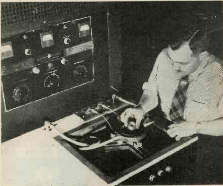
Operator placing small gear in fixture preparatory to inductive heating for surface hardening with G-E 15 kw electronic heater
