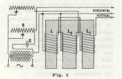
Two identical coils L and L¹ having a great many turns (say several thousand), are inserted on the outer legs. They should be tightfitting. Windings from two highresistance chokes, such as the replacement components for small acdc receivers provide satisfactory coils here. The center leg can be a similar winding or a larger one but should fit the center leg rather tightly.
