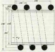
Fig. 2. Three turn wire - wound coil
