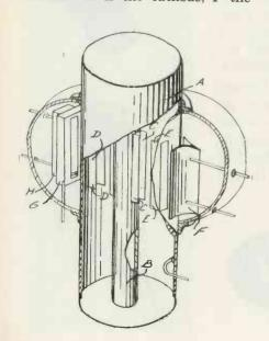
collector anode. The electron stream is velocity-modulated in the gap between D and C, it becomes bunched during passage through C and transfers energy to the resonator when traversing the space between C and E. For tuning, the length of the resonator can be made adjustable. Several sets of slots, either parallel or obliquely arranged, may be provided. J. H. Fremlin, International Standard Electric Corp., (F) Nov. 27, 1940, (I) June 1, 1943, No. 2,320,860.
