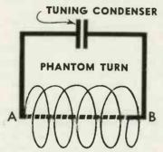
Fig. 7. Showing effect of lend connections external to the coil
