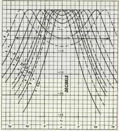
Fig. 2. Here the scale of abscissae is pure number: that is, units of p=1/Q. To convert to frequency, multiply by fo. For example, if the Q of the coils is 20, and the center-frequency is fo=10 mc, then each division (p) represents  $pf_0$  cycles=0.05x10 mc=500 kc
