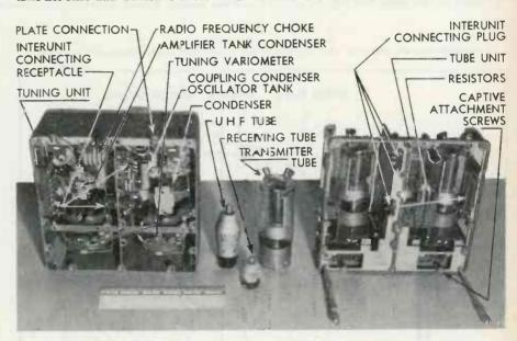
TRANSMITTERS for long and short waves are mopa, identical except for frequency
