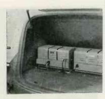
Complete 22 Watt High Frequency Mobile Installation
