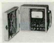
high degree of accuracy both as a resistance measuring instrument and as an insulation tester. Housed in a heavy-duty oak portable cabinet with a bakelite panel the device measures  $9\frac{1}{2} \times 8\frac{1}{2} \times 6$  in. When battery operated, the 500 v. potential is made available by means of an integral vibrator power supply by throwing a front panel toggle switch. Price \$62.50. Another model, 610-E, operates on 110 v. ac and is available for \$52.50.
