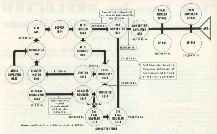
BLOCK diagram of the 25-watt General Electric transmitter showing manner in which crystal and master oscillator frequencies are combined and eventually produce the final operating frequency of 330.45 megacycles
