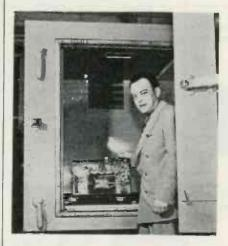
R. H. FRYE, chief engineer, Electronic Laboratories, Inc., Indianapolis, determines whether a power supply unit will work in any weather by testing it under operating conditions in new temperature, humidity and altitude chamber
