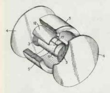
of the cycle, but electrons continuously withdrawn from cathode 12 are stored up within cylinder 11 as rotating space charge and are extracted as they are needed by the main oscillating circuit. W. T. Gibson, International Standard Electric Corp., (F) May 8, 1940, (I) July 20, 1943, No. 2,324,772.
