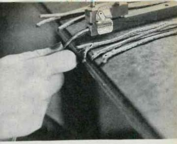
SHIELDING STRIPPER cuts time of operation from 55 seconds to 15 seconds at Submarine Signal Co., Boston, Mass. Wire is inserted, then pulled out. Pawl-action knife cuts metal braid. Screws adjust for length and depth of cut
