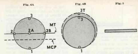
Illustrating current distribution in wire and in strap conductors at high frequencies
