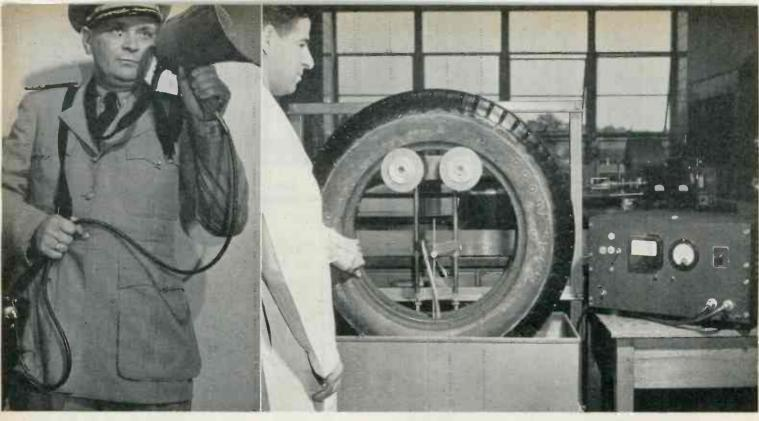
P.A. MEGAPHONE for use on merchant vessels, made by Guided Radio Corp., V. Y. Mike and speaker in megaphone, amplifier slung over shoulder
