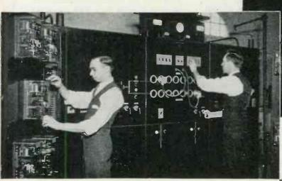
CARRIER - CURRENT laboratory containing complete replica of high tension transmission lines
