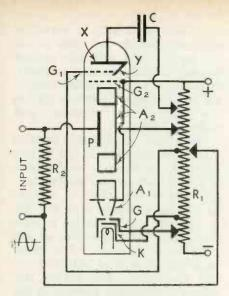
Fig. 6. Scanning wave generator directly synchronized
