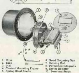
The new 400 cycle meter, like all other J-B-T Vibrating Reed Frequency Meters, requires no adjustment while in service, even under adverse vibration conditions. It is not affected by wave form, normal temperature changes or external magnetic fields. Simply READ the REED and that's your frequency.
