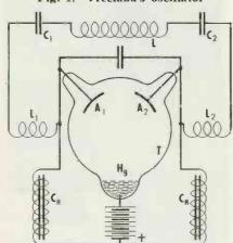
determined by these constants. Stable operation is aided by the inductive chokes in the anode supply leads, shown as  $C_{\rm H}$ . The Vreeland tube is thus, basically, a synchronous switch.
