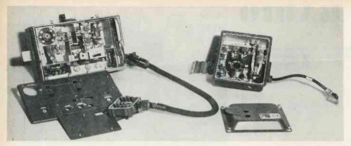
BLIND landing equipment used on the Messerschmitt Me 110 fighter plane operates on the Lorentz system and consists of two units, the beacon receiver and the marker beacon receiver, both operating through a common audio amplifier
