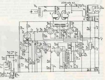
WELDER control circuit adjustable between one half-cycle and 60 half-cycles
