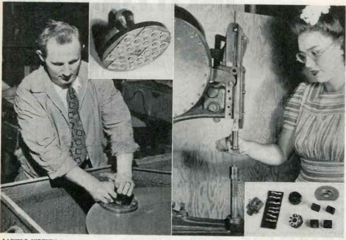
LAPPING FIXTURE holds twelve electrodes. By adopting technic used to lap crystals themselves, RCA Canden plant cuts electrode lapping time to 0.8 minutes from old handlapping time of 2.0 minutes each. Close-up at top right
