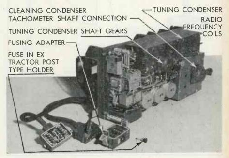
RADIO compass receiver is trf unit covering two bands for aural and visual use
