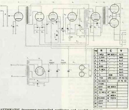
AUTOMATIC frequency-controlled oscillator and amplifier circuit
