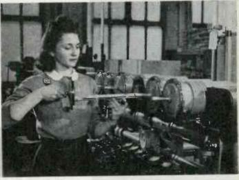
SILVER SUBLIMATION method efficiently plates quartz crystals in Western Electric Chicago works. Operator inserts tray of finished blanks into vacuum chamber for evaporation and deposition of protective silver film
