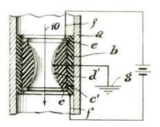
varnish is obtained. 10 indicates the electron path. Bushing c' and coating d' may be of suitable shape and thickness to provide a desired electric field. F. Krause, Alien Property Custodian, (F) Dec. 2, 1940, (I) March 2, 1943, No. 2,313,-018.
