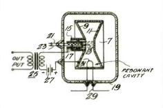
shown, the cavity electrode is maintained at a positive potential and serves as anode. Distance between cathode and effective anode must be such that the electron transit time is less than a half period. E. G. Linder, RCA, (F) June 25, 1940, (I) March 23, 1943, No. 2,314,794.
