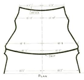
EXPONENTIAL-HORN FORM given the stage section is eterrty shown in both sketches and photographs. These also reveat details of the 2-ton curved "drop" which can be lowered to cut off the backstage, when entire space is not needed for a 125-piece orchestra
