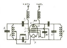
tralizing capacity NC may be inserted. The oscillations generated may be modulated by applying potentials to grid 1, grid 2 or to plate AN. Alan D'Arcy Hodgson, RCA, (F) Oct. 10, 1931, (I) March 9, 1943, No. 2,313,071.
