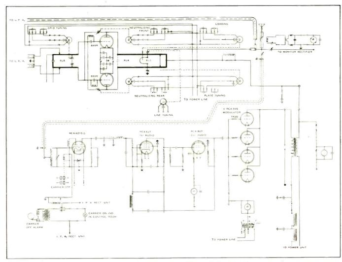
FINAL RF POWER AMPLIFIER with an automatic monitoring system that balances out any amplitude modulation products that may be present
