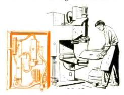
Accurate Welding Control—The use of small Ignitron tubes has practically eliminated mechanical contacts for resistance welding. In the Westinghouse power switch, Weld-O-Trol, action is instantaneous. Speed of current interruption is 600 or more times per minute. The two Ignitron tubes in each Weld-O-Trol are guaranteed for a year and have consistently held up for much longer periods.
