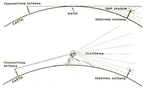
HOW THE RANGE OF A UHF station is affected by terrain. Above, the range is simply optical plus ten per cent for bending. The shadow is so pronounced that almost not a signal is heard below horizon, regardless of power of transmitter. Below, the range is indefinite, as the signal is scattered by trees and wires on top of the hill. Of course, much weakened signals result, but the coverage is larger than over the water
