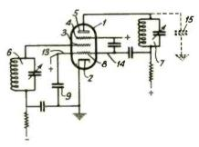
and to the output electrode via lead 14. In a preferred embodiment, cathode 2 is connected to the anode side of suction grid 8 instead of to its control grid side. G. H. P. Alma, M. J. O. Strutt and A. van der Ziel, Alien Property Custodian, (F) May 9, 1941, (I) March 30, 1943, No. 2,314,916.
