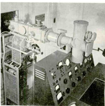
IFDIVIBUAL LABORATORIES are completely empipped for the insessignation of particular projects. In the cas above, an investignation of the physical properties of rubber is under way. Tersile, compression and plasticity tests are conducted here on rubber compounts under controlled temperature and hereidits conditions.
