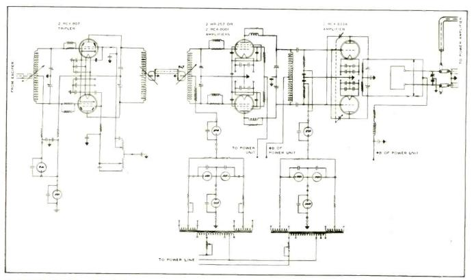
INTERMEDIATE RE AMPLIFIER increases the power level and triples the frequency
