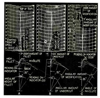
HIGH FILLET, underent and tip modification as charted on electrical recorder
