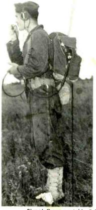
Signal Corps portable field transmitter-receiver in use
