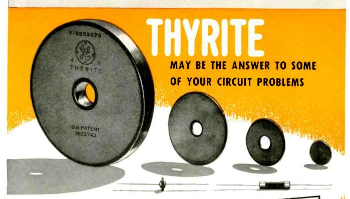
THYRITE\* is a silicon-carbide ceramic material, dense and mechanically strong, having nonlinear resistance characteristics—the resistance varying as a power of the applied voltage. Its resistance characteristic is stable, and substantially independent of polarity or frequency. Thyrite has been used for many years in many important applications, including electronic. Thyrite can be produced in various shapes and sizes (those which can be successfully molded).
