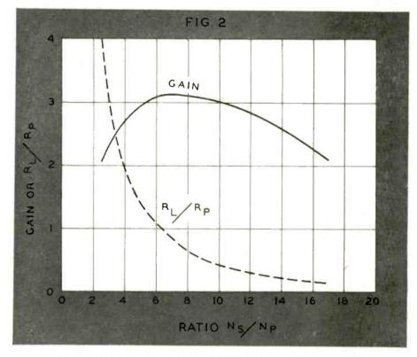
Fig. 2. Each special purpose transformer has its own turn-ratio optimum
