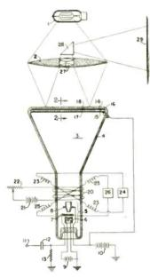
when the dispersion of the paraffin layer is a minimum and decreases with increasing dispersion. The dispersion of paraffin is dependent on its temperature which in turn is controlled by the amount of electrons impinging on the paraffin layer. The scanning beam is modulated with picture signals and deflected in a conventional manner. P. T. Farnsworth, Farnsworth Television and Radio Corp., (F) Sept. 7, 1940, (I) March 30, 1943, No. 2,315,-113.
