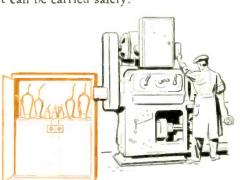
Speed Control—By converting a-c power to direct current with thyratron tubes, Westinghouse has developed small, compact speed control units for d-c motors without using rotating equipment for current supply. Direct current is supplied by the tubes to the armature and field of the d-c motor. Both armature and field circuits are controlled by one dial on the Westinghouse Mot-O-Trol.
