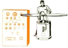
Vibration Fatigue Tests—Only through electronics has it been possible to build vibration testing equipment that will deliver from 10 to 10,000 cycles per second. Employing the principle of the dynamic radio speaker, Westinghouse engineers have developed vibration fatigue equipment that has opened the way for tests that could not be made with existing mechanical methods.
