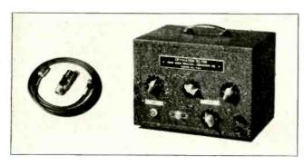
Fig. 2. A selective amplifier developed by Rowe Radio Research Laboratory, 2422 N. Pulaski Rd., Chicago, for automotive engine studies
