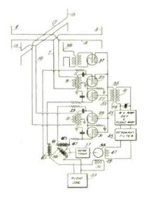
move. If the received waves do not apply equal currents to the antennas, unequally modulated components will modulate the carrier and will be applied to the receiver which, upon demodulation, will cause rotation of rotor 55 until equal and opposite modulation components are produced in the pairs of balanced modulators 25, 27 and 29, 31. The bearing of the waves will be indicated by pointer 67. V. D. Landon, RCA, (F) June 28, 1940, (I) March 16, 1943, No. 2,314,-093.
