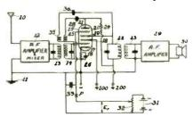
such a way as to keep amplification constant. An inverse feedback circuit deriving its potential from anode 19 may be added. The potential of control grid 20 can be supplied by a rectified output signal, e.g., if pass range adjustment for control of background noise or needle scratch suppression is desired. H. Boucke, Patents Research Corp., (F) March 29, 1940, (I) March 30, 1943, No. 2,315,043.
