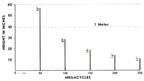
HOW THE ENERGY intercepted by a quarter-wave antenna decreases as the frequency goes up, based on the fact that a transmitter lays down a signal in microvolts per meter
