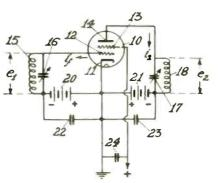
14, or, under certain provisions, by modulating the screen grid voltage. Various applications of this principle to beat-frequency oscillators, superheterodyne receivers and transmitters are described. H. M. Bach, Patents Research Corp., (F) Aug. 22, 1940, (I) Feb. 23, 1943, No. 2,311,631.
