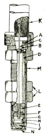
Fig. 3. A piezo pressure gage for cylinder combustion measurements
