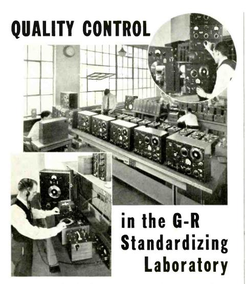
However well designed an instrument may be, accurate calibration and reliability in service determine its ultimate usefulness. Testing, therefore, has long been an important final step of our manufacturing; approximately 10% of the total man hours required to produce a General Radio instrument is spent in our standardizing laboratory. Here a carefully planned schedule of tests and measurements transforms an unadjusted, uncalibrated device into a precision instrument.
