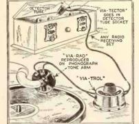
This illustration shows the units and connections of the Via-Rad reproducer and the simplicity of the entire arrangement. Via-Rad is a proven B.M.S. product that can be quickly attached, without tools, to any phonograph to change the phonograph into a radio operated instrument of unsurpassed quality for the true and life-like reproduction of voice and music.
