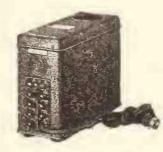
"B"POWER UNIT. Automatically controlled by switch on receiving set. "A" battery and trickle charger can be connected to this "B" Power Unit, in which case the automatic switch also starts and stops charger, if one is used. Plugs into A.C. light socket. Delivers up to 135 volts. Operates Atwater Kent Receivers or other make consuming not more than 40 milliamperes. Brown crystalline finish. Including long-life rectifying tube (no filament to burn out) and 7-foot flexible cord.
