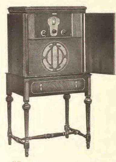
6K The model illustrated is the Kolster full console 6 tube electric set. Cabinet of walnut with special builtin cone speaker. This set operates from any 110 volt 60 cycle electric line. The tubes used in this set are as follows: four UX 226 or CX 326, one UY 227 or C 327, one UX 171 or CX 371, one UX 280 or CX 380. Price, \$250. Tubes extra.
