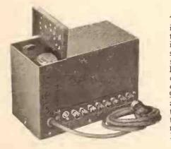
The National "B" Eliminator is unquestionably NATIONAL BATTERY ·B" the outstanding Elim inator on the market this season. Operates on any set using 201A tubes or Power tubes. Has only one dial-simple and easy to operate. Taps for 45-671/2-90-135 and 180 volts. Can also be used with any Na-tional Homepower Unit to give a compact, auto-matic, efficient "A B" matic, efficient Power supply.
