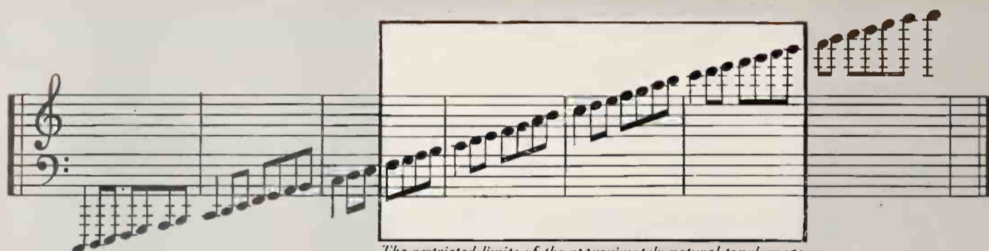
The restricted limits of the approximately natural tonal range of the phonograph, represented diagrammatically.
