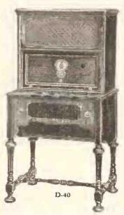
D-40 Five tubes. Wet or dry battery type. Balanced, tuned radio frequency. Centralized control. Built-in speaker. Latest acoustical design. Deep, rich tone quality. Receiver compartment slides out to install tubes. Genuine walnut cabinet. Ample space for all batteries.
