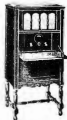
MAGNAVOX 75 Five tube tuned radio frequency set. Built-in Magnavox Loud Speaker; encloses all batteries. Artistic mahogany cabinet, hand rubbed finish. Price, without tubes or batteries, $200
