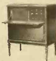
B-35 Five tubes—199's or 201-A's. Balanced tuned radio frequency. Delicate parts completely shielded. Apparatus slides out to install tubes. Beautiful cabinet of selected mahogany, finished in rich two-toned effect. Exceptional enclosed speaker. Ample space for all batteries. Length 35 inches, height 23 inches, depth 21 inches. Price, without accessories $250.00
