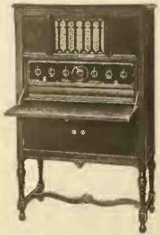
THERMIODYNE—MODEL CTF6—CONSOLE DE LUXE Model TF6, enclosed in Console Cabinet of genuine Walnut, with built-in Loud-Spacker, and with space for Batteries and Charger. All equipment concealed. No wires required for local stations.
