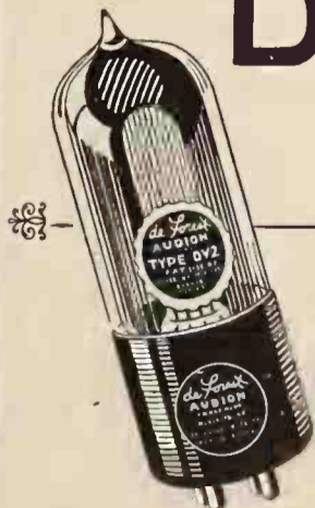
The DV-2 has a filament potential of 4½ volts and a filament consumption of 25/100 of an ampere.
