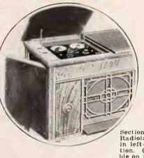
Sectional view of cabinet showing Radiola Super-Heterodyne installation in left-hand top convenient to operation. (Phonograph equipment available on right-hand top side of cabinet.) No outside wires required. Large dlrectional loop has been installed in swinging left-hand END PANEL of cabinet.
