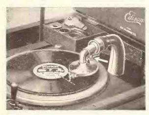
SHOWING POSITION FOR PLAYING EDISON OR OTHER HILL AND DALE CUT RECORDS Turn reproducer to play Edison or other hill and dale cut records and the weight of reproducer is automatically decreased to the Edison weight, the needle is centered and the reproducer assumes the flat or Edison position.
