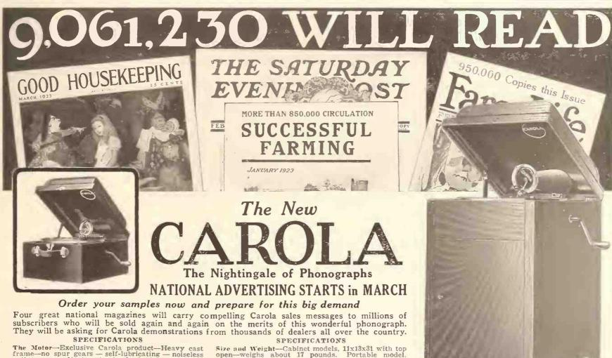
The Motor—Exclusive Carola product—Heavy cast frame—no spur gears—self-lubricating—noiseless action—easy adjustment—standard 14-foot spring—plays full 12-inch record one winding—used on all new Carola models.
