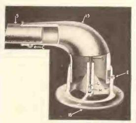
No. 16—Base. No. 15—Large Elbow. No. 5—Adjustable length extension. M—Screw for adjusting height of Tone Arms. L—Ball-bearing, insuring extremely sensitive swing to Tone Arm. S—Fixed stud in Large Elbow. E—Stop screw for swing or are of Arm. This screw also holds Base to Large Elbow.
