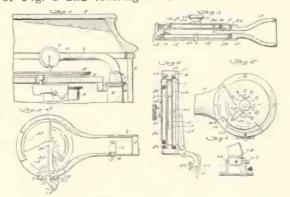
arrows; Fig. 5 is an enlarged rear elevation of the sound box shown in Fig. 1, the back of the sound box being broken away to show the structure contained therein; and Fig. 6 is an enlarged detail view partly in vertical section and partly in elevation, showing the mounting of the tone arm.
