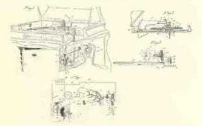
left side elevation and partly in vertical section taken through the cabinet at the axis of the turntable; Fig. 3 is a front elevation of certain of the parts shown in Fig. 2, with some parts shown in different positions by means of broken lines; and Fig. 4 is a view showing the wiring diagram for the repeater.
