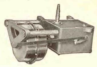
1. The wick lubricating system, an exclusive feature of our motor, keeps every part in the gear box running in a film of oil. Not a mere smear of grease to dry away and get gummy and hard with exposure to the air, causing noise and variable speed within a short space of time, but constant circulating lubrication.
