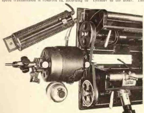
Duplex Phonograph Recorder for Radio Signals in Use at the New York Times Radio Station In New York City. The Second Record Can be Started While the First Is Still Rotating, so as to the Machine which Obtain a Continuous Record of Long Incoming Messages. Signals Can Also be Recorded on the Records at High Speed, and Afterwards Transcribed on a Low Speed Phonograph.
