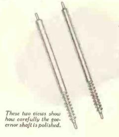
After the governor shaft is made, it is polished by drilling it hundreds of times in a piece of maple. Every burr is removed and the shaft, when finished and buffed, leels smooth as velvet and glistens like silver. A man can polish only about 100 shafts a day.
