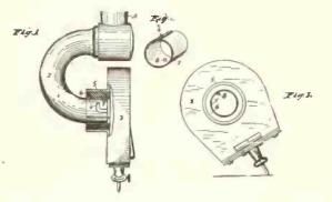
box. Fig. 2 is a perspective view of the split ring. Fig. 3 is a side elevation, showing the rear side of the tone box and the connection between the tone arm and the sound box.
