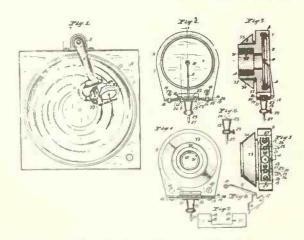
section on line 3—3 of Fig. 2. Fig. 4 is a rear view of the reproducer. Fig. 5 is a bottom view of the same. Fig. 6 is a side elevation of the stylus holder. Fig. 7 is a plan view of the bear-
