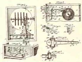
machine of Fig. 1, certain of its component instrumentalities being shown in side elevation. Fig. 3 is a fragmentary side view upon an enlarged scale of one group of records partly in section and partly in elevation, the sight being taken on the dotted line 3—3 of Fig. 1. Fig. 4 is a fragmentary end elevation on the line 4—4 of Fig. 2; and Fig. 5 is a fragmentary side view of a modification.
