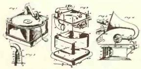
away, of the horn form of the machine; and Fig. 5 is a perspective view of the bracket and rod or wire for mounting the tone arm and horn.
