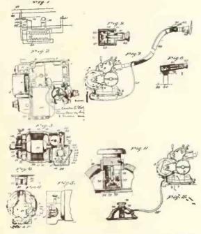
vention and illustrating a start-and-stop device therefor in the form of a foot-controlled switch, the latter being shown in enlarged vertical section; and Fig. 11 is a further enlarged vertical section of the switch of Fig. 10 at right angles to the section of the latter figure.
