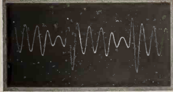
No. 3.—French Horn.—Here is another instrument with a smooth, more or less fluent tone, though quite different in quality from that of the violin. From the appearance of its tone waves, one might almost anticipate the rounded mellow beauty of this instrument.
