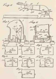
arm at the vertical plane of the axis about which it swings horizontally. Fig. 2 is a section at the line, 2—2, on Fig. 1. Fig. 3 is a detail side elevation of the elbow portion of the tone arm, showing an exteriorly-accessible device for adjusting the tension of the counter-balancing spring.
