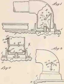
its mounting, particularly with respect to its connections for swinging over the record and toward and from the record, and for counterbalancing any excess of weight of the tone arm causing undue pressure of the stylus upon the record
