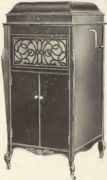
Model 250—Retail at $200. Finish: Mahogany, light, dark and natural wood colors. Motor: No. 16 Meisselbach, playing five ten-inch records with one winding. Dimensions: Height, 51½ inches; width, 23 inches; depth, 25½ inches. Universal tone-arm. Automatic stop. All metal parts gold or nickel-plated.
