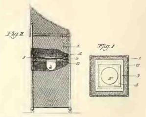
the central portion of said cabinet, showing the motor and turn table mounted on a plaited non-resonant ledge. Fig. 2 shows a side elevation of the new talking machine cabinet, partly in section, showing a motor and turn table mounted thereon.
