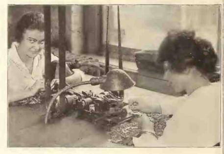
Showing details of pointing machine into which one needle, at a time, is fed.
