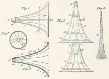
horn, while a large part of its longitudinal extension must be bent in the transverse direction to secure the flare of the horn. This double or transverse bending of a normally flat piece of wood sets up internal stress in each strip of wood, tending to cause\_said strips to return to their normal flat condition. This tendency, if not counteracted, would result in separation of the strips forming a horn of the bell or flaring shape.
